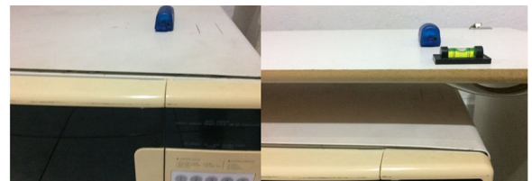
Fig. 4 Photos of the measurements using an accelerometer placed directly over the microwave oven top (left) and placed on the shelf (right)
