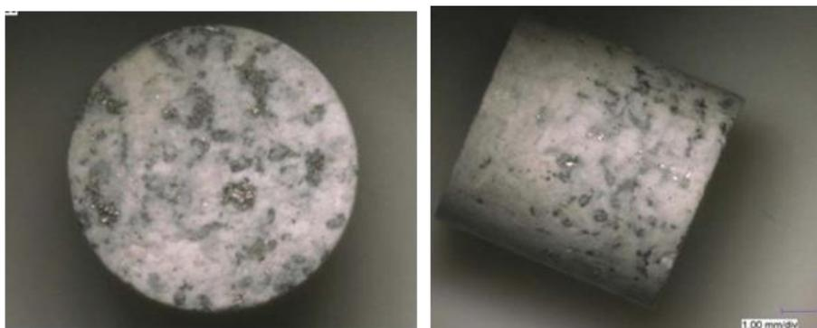
Figure A.1. Pilot-plant pellets 6x6 mm, 5% ENG, density of .391 g/cc with standard deviation of  $0.013 \text{ g/cm}^3$ . Both top view (left) and side view (right) are shown here.
