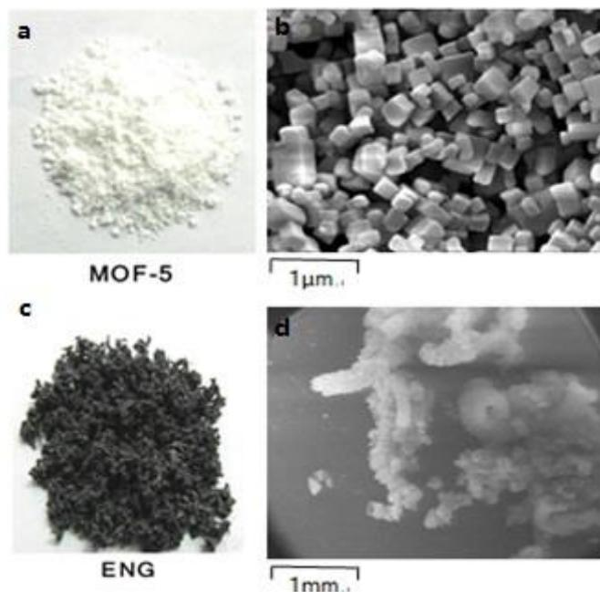
Figure 4.1. Images of MOF-5 (upper panel) and ENG powders (lower panel).
