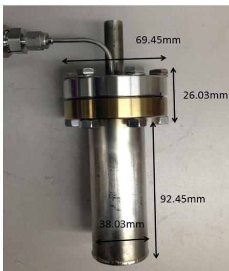
Figure 8.2. Picture of vessel used in NIST neutron imaging experiment. Dimensions are shown in the graph.
