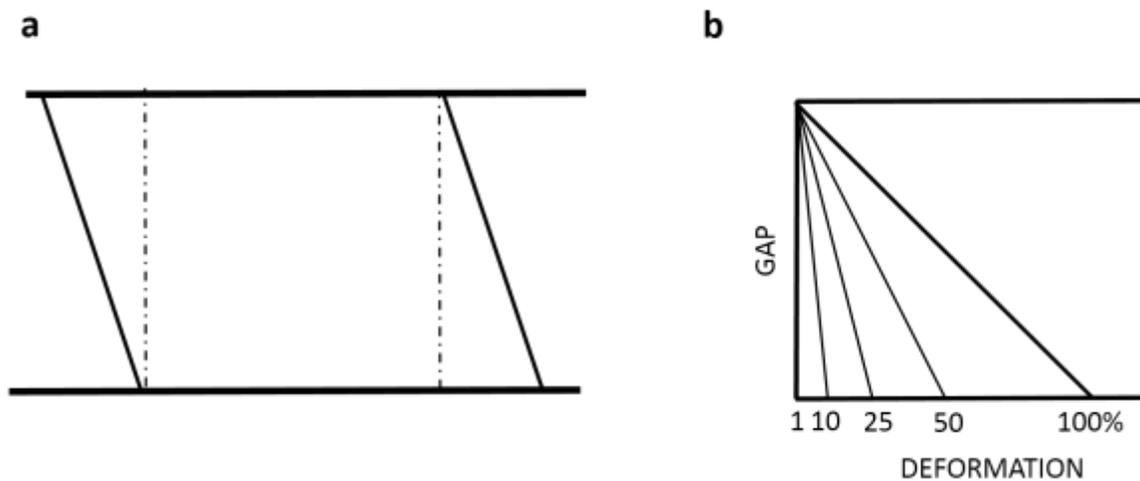
*Figure 5. Illustrations of shear strain a) effect of shearing by lower plate b) large shear strain results in larger deformation and stretching near the edges of the plate.*
