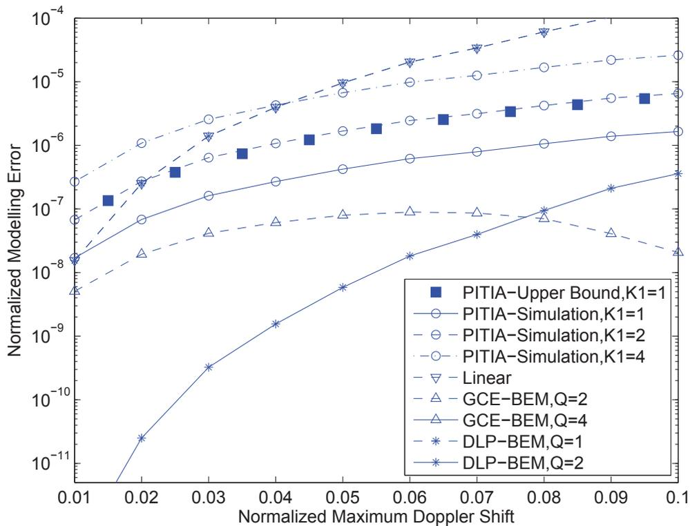
Figure 3.6: Modelling errors of PITIA, piece-wise linear approximation, GCE-BEM and DLP-BEM, with  $N = 2048$  and  $L = 16$ ; the curve labelled with “linear” denotes “piece-wise linear approximation”.
