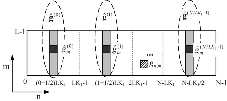
Figure 3.2: The basic principle of PITIA: the time varying channel  $g_{n,m}$  is approximated by a series of  $\hat{\mathbf{g}}^{(u)}$
