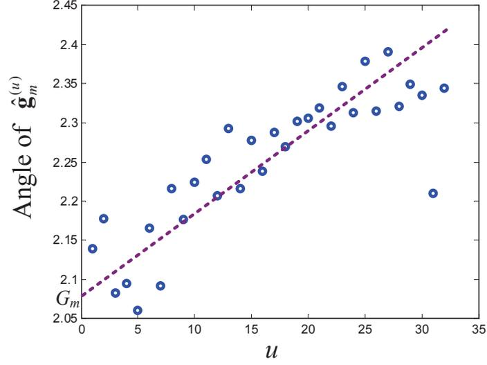
Figure 3.4: Phases of  $\hat{\mathbf{g}}_m^{(u)}$  for  $u = 0, 1, \dots, N/LK_1 - 1$ ; the phase of  $g_m$  and the Doppler shift  $\delta_m$  are derived from the start point  $G_m$  and the slope of the dashed straight line that fits all the data points with least squares approach, respectively.
