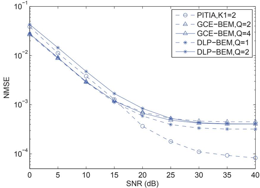
Figure 3.10: NMSE of the proposed algorithm, piece-wise linear approximation, GCE-BEM and DLP-BEM, with  $N = 2048$  and  $L = 16$ ; “ground truth” of the wireless channel is simulated by WINNER II, and  $f_{max}$  is around 841 Hz.
