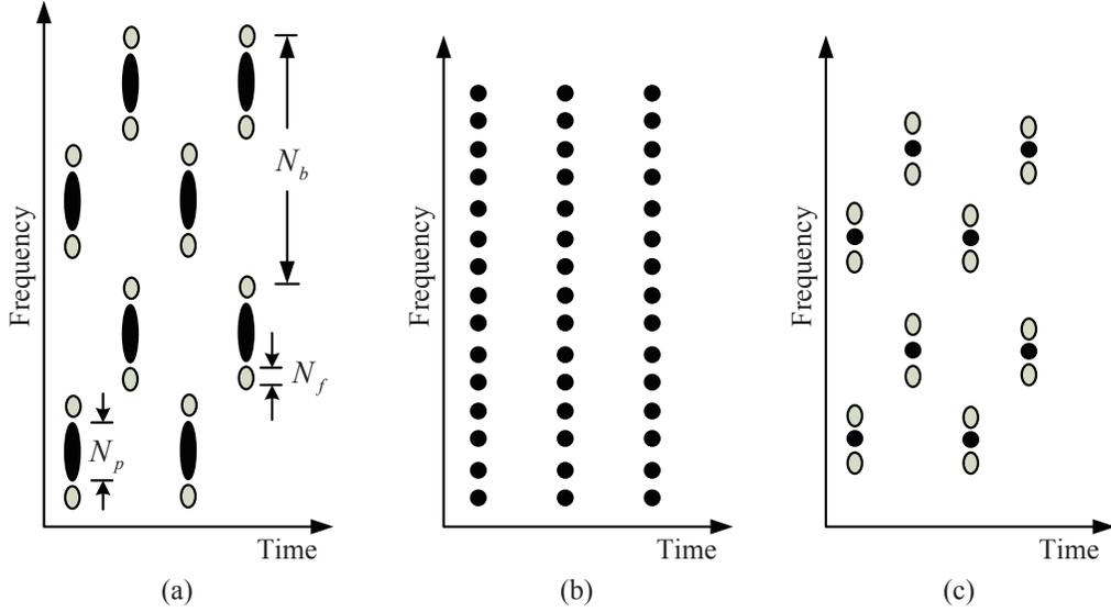
Figure 3.3: Comb-type (a), block type (b) and FDKD (c) pilot allocation schemes
