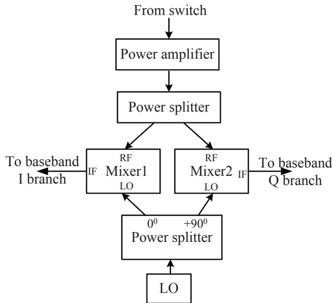
Figure 4.9: Receiver branch of RF circuits designed by discrete RF components
