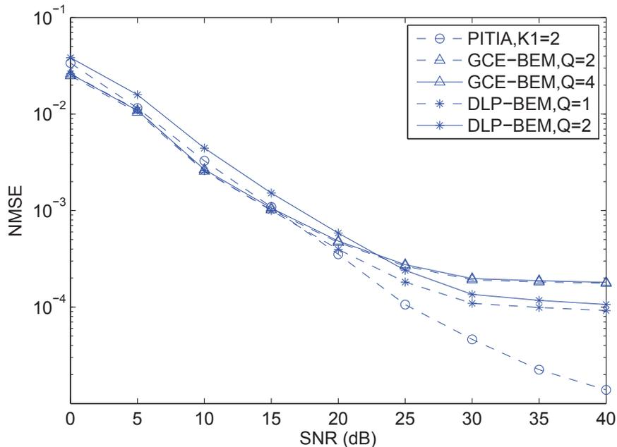
Figure 3.11: NMSE of the proposed algorithm, piece-wise linear approximation, GCE-BEM and DLP-BEM, with  $N = 2048$  and  $L = 16$ ; “ground truth” of the wireless channel is simulated by WINNER II, and  $f_{max}$  is around 361 Hz.
