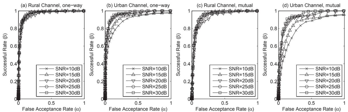
Figure 4.7: ROC curves of PHY-CRAM for one-way (a)(b) and mutual (c)(d) authentication under rural channel (a)(c) and urban channel (b)(d) derived by simulation, with key length  $M = 60$
