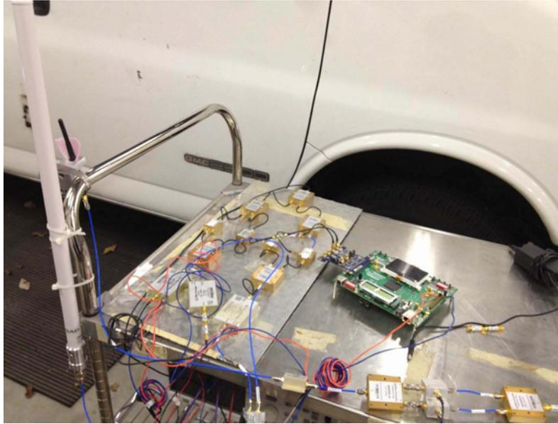
Figure 2.3: The photo of the FPGA-based prototype for PHY-CRAM
