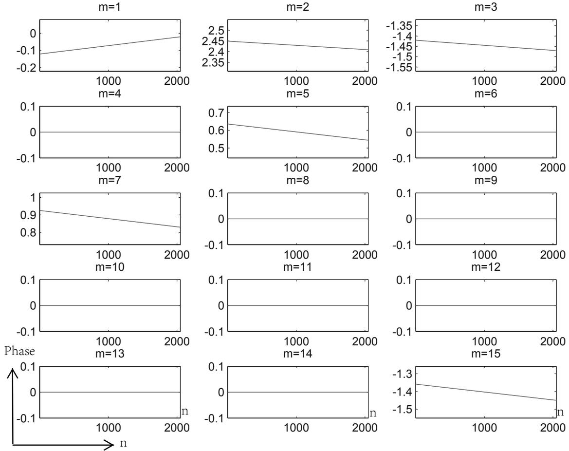
Figure 3.1: Phases of the time-varying channel response on channel taps 1 to 8 derived from WINNER II channel model; x-coordinate denotes  $n$  while y-coordinate denotes the phase of  $g(n, m)$  for a given number of  $m$
