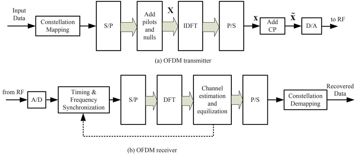
Figure 2.1: The block diagram of an OFDM system
