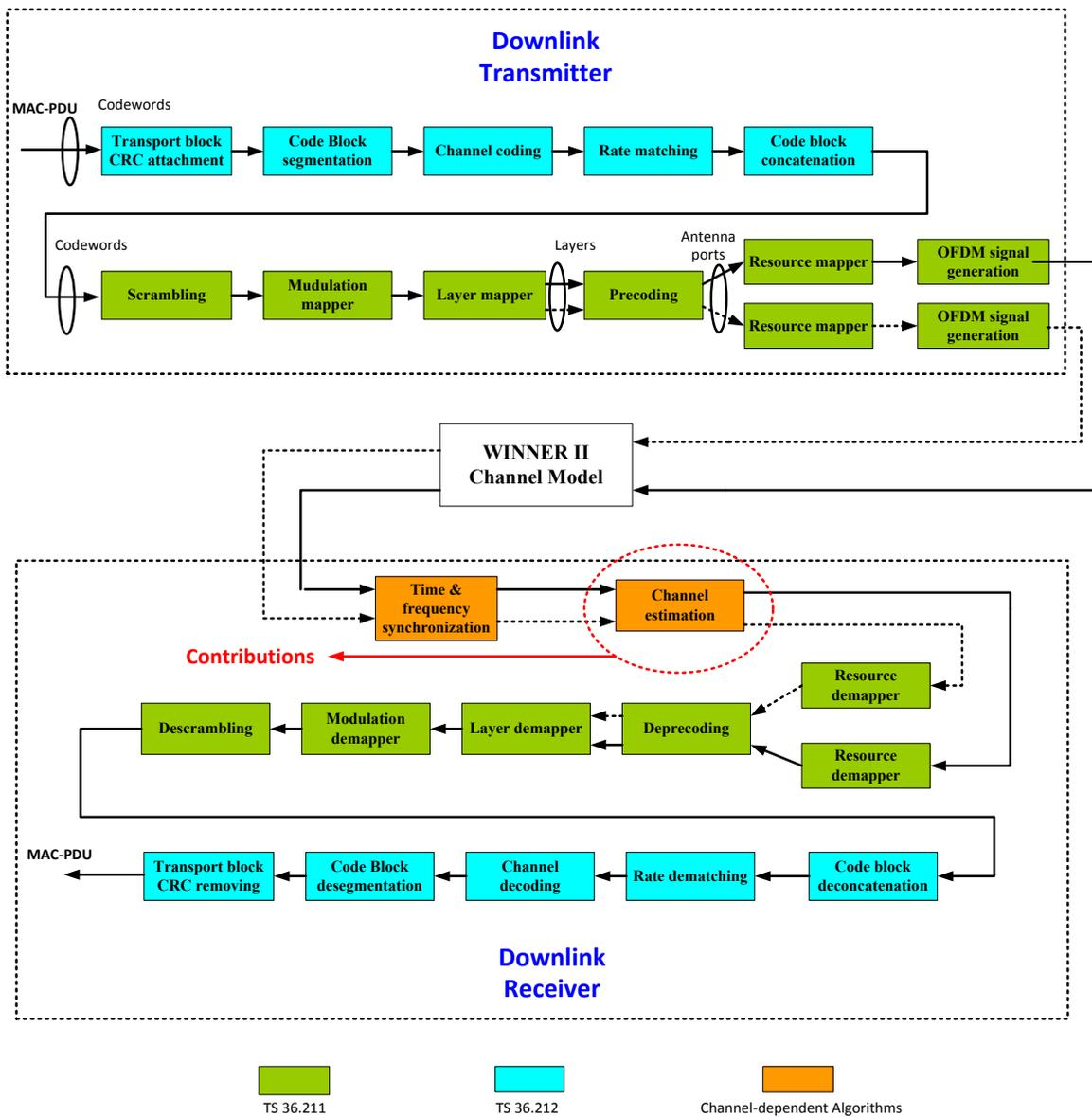
Figure 2.2: The block diagram of a LTE simulator developed to evaluate the performance of PITIA
