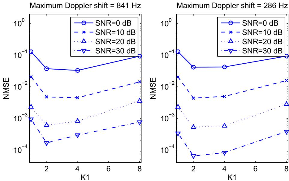
Figure 3.7: NMSE changes over  $K_1$  under different SNR and Doppler shift conditions
