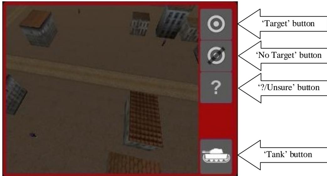
*Figure 4-5: One of the nine UAV feeds with associated response buttons*
