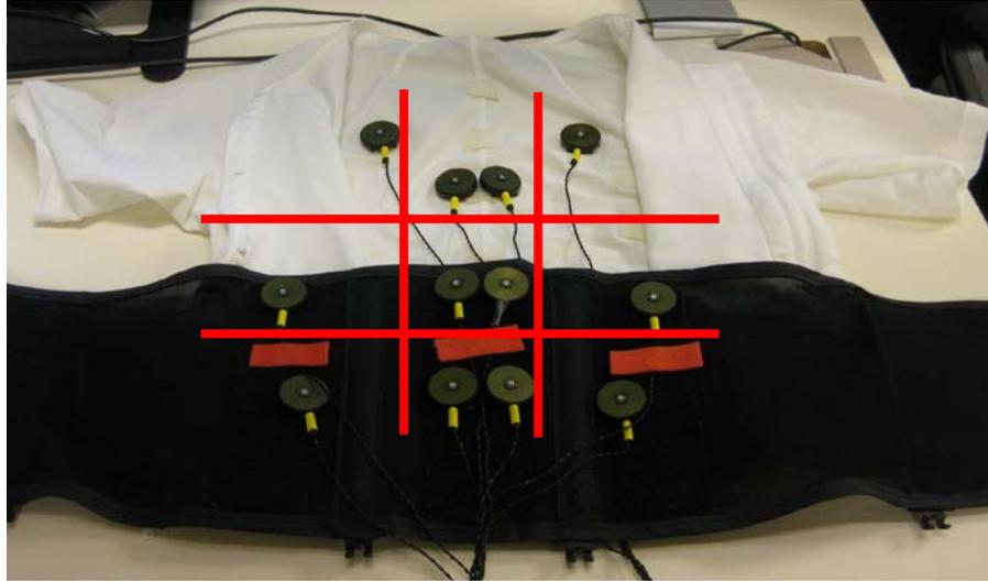
*Figure 2-3: Tactor vest (top) and belt (bottom), with 12 tactors divided over 9 sectors to map onto the 9 UAV feeds on the monitor*
