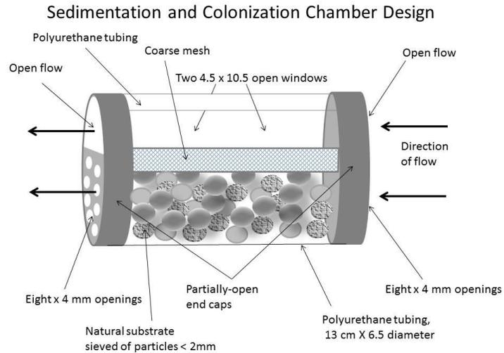
Fig. 1: Sedimentation and colonization chambers were designed to create an open flow habitat to allow both particles and invertebrates to enter the chamber. The natural substrate was collected on site and sieved to remove particles less than 2 mm. Design follows a similar technique as Korchersberger *et al.* (2012).
