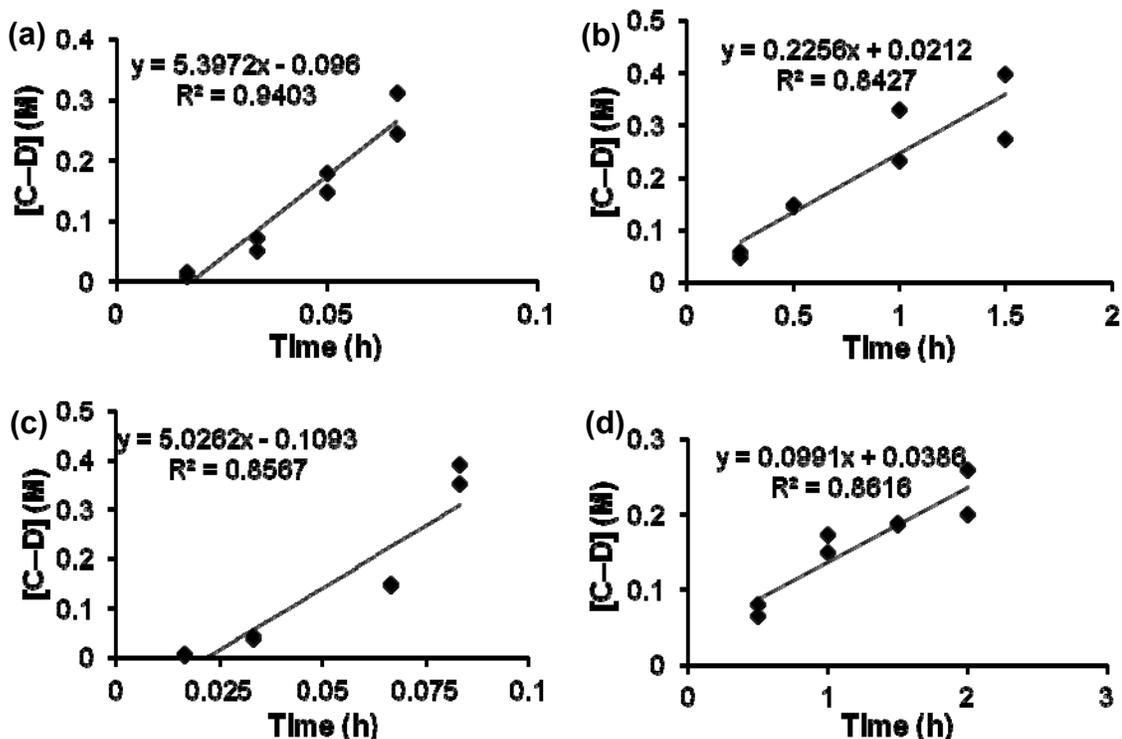
Conditions: (a) and (b): Pt<sup>II</sup> catalyst (2 mol %, 5  $\mu$ mol), benzene (23.2  $\mu$ L, 0.26 mmol), AgOAc (1.7 mg, 10  $\mu$ mol) in CF<sub>3</sub>CO<sub>2</sub>D (0.5 mL, 6.5 mmol, 25 equiv relative to benzene) at 150 °C. (c) and (d): Pt<sup>II</sup> catalyst (2 mol %, 5  $\mu$ mol), benzene (23.2  $\mu$ L, 0.26 mmol), AgBF<sub>4</sub> (1.9 mg, 10  $\mu$ mol) in CD<sub>3</sub>CO<sub>2</sub>D (0.37 mL, 6.5 mmol, 25 equiv relative to benzene) at 150 °C.
