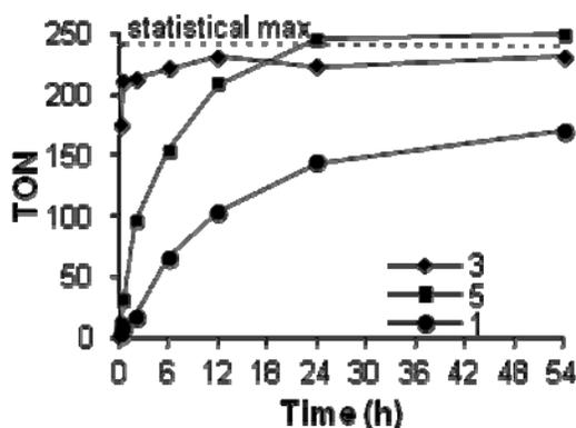
Conditions: Pt<sup>II</sup> catalyst (2 mol %, 5 μmol), benzene (23.2 μL, 0.26 mmol), AgBF<sub>4</sub> (1.9 mg, 10 μmol) in CD<sub>3</sub>CO<sub>2</sub>D (0.37 mL, 6.5 mmol, 25 equiv relative to benzene) at 150 °C.
