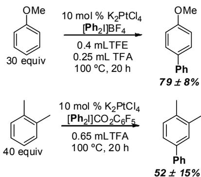
Conditions: Catalyst (0.93  $\mu$ mol, 10 mol %), arene (2.7 mmol, 30 equiv),  $[Ph_2]X$  (0.093 mmol, 1 equiv) in the designated solvent (0.65 mL) at 100 °C for 20 h. Calibrated yield and selectivity determined by GC.
