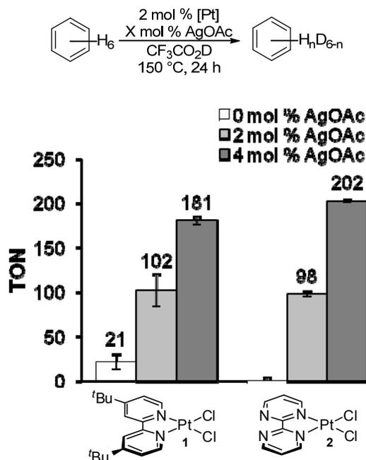
Conditions:  $\text{Pt}^{\text{II}}$  catalyst (2 mol %, 5  $\mu\text{mol}$ ), benzene (23.2  $\mu\text{L}$ , 0.26 mmol), AgOAc (1 equiv, 0.85 mg, 5  $\mu\text{mol}$ ; 2 equiv, 1.7 mg, 10  $\mu\text{mol}$ ) in  $\text{CF}_3\text{CO}_2\text{D}$  (0.5 mL, 6.5 mmol, 25 equiv relative to benzene) at 150 °C for 24 h. Reported as TON  $\pm$  standard deviation.
