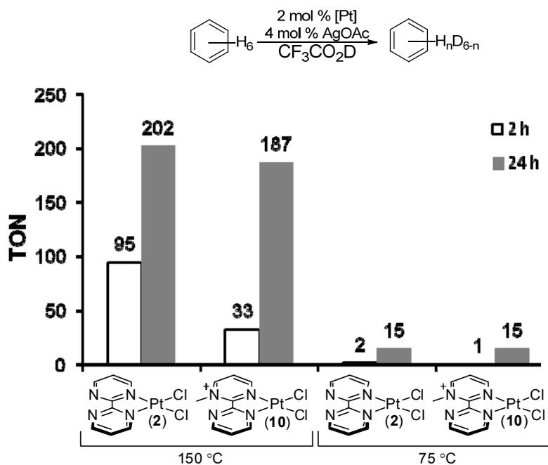
Conditions: Pt<sup>II</sup> catalyst (2 mol %, 5 μmol), benzene (23.2 μL, 0.26 mmol), AgOAc (1 equiv, 0.85 mg, 5 μmol; 2 equiv, 1.7 mg, 10 μmol) in CF<sub>3</sub>CO<sub>2</sub>D (0.5 mL, 6.5 mmol, 25 equiv relative to benzene) at 75 or 150 °C for 2 or 24 h. Reported TONs are the average of at least two trials.
