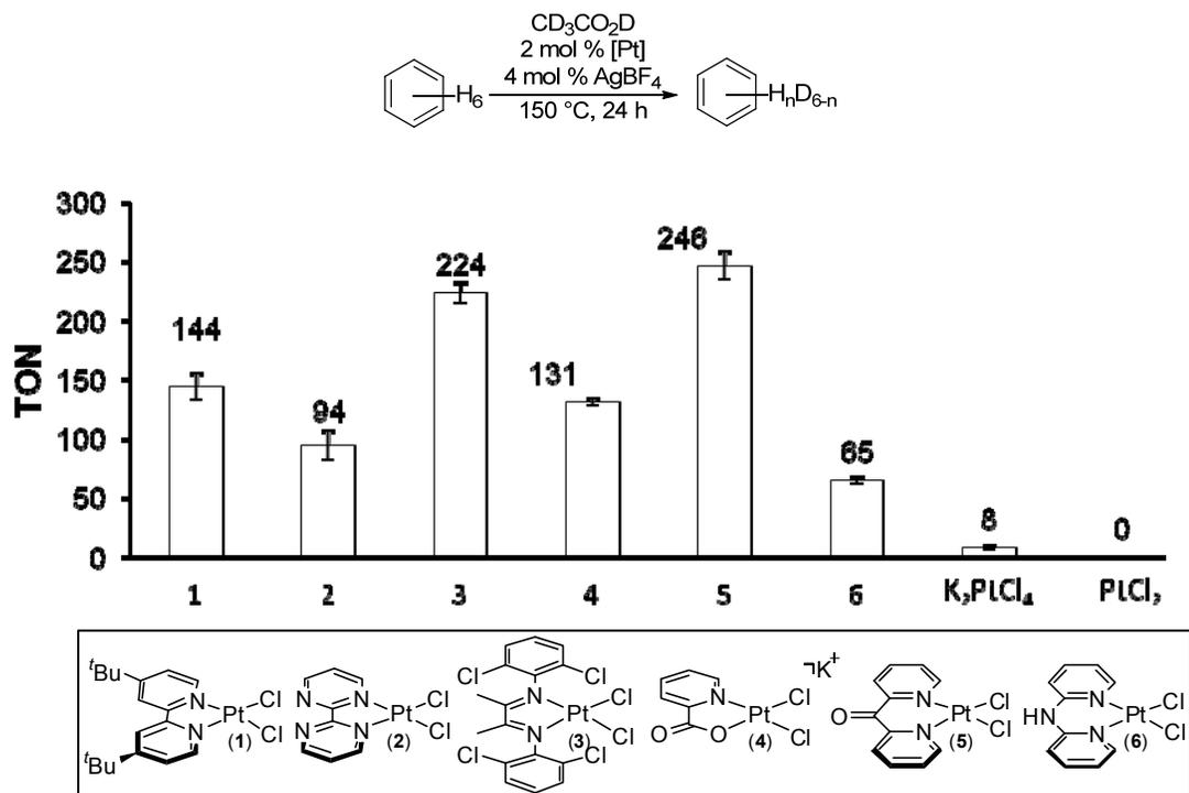
Conditions:  $\text{Pt}^{\text{II}}$  catalyst (2 mol %, 5  $\mu\text{mol}$ ), benzene (23.2  $\mu\text{L}$ , 0.26 mmol),  $\text{AgBF}_4$  (1.9 mg, 10  $\mu\text{mol}$ ) in  $\text{CD}_3\text{CO}_2\text{D}$  (0.37 mL, 6.5 mmol, 25 equiv relative to benzene) at 150  $^\circ\text{C}$  for 24 h. Reported as TON  $\pm$  standard deviation.
