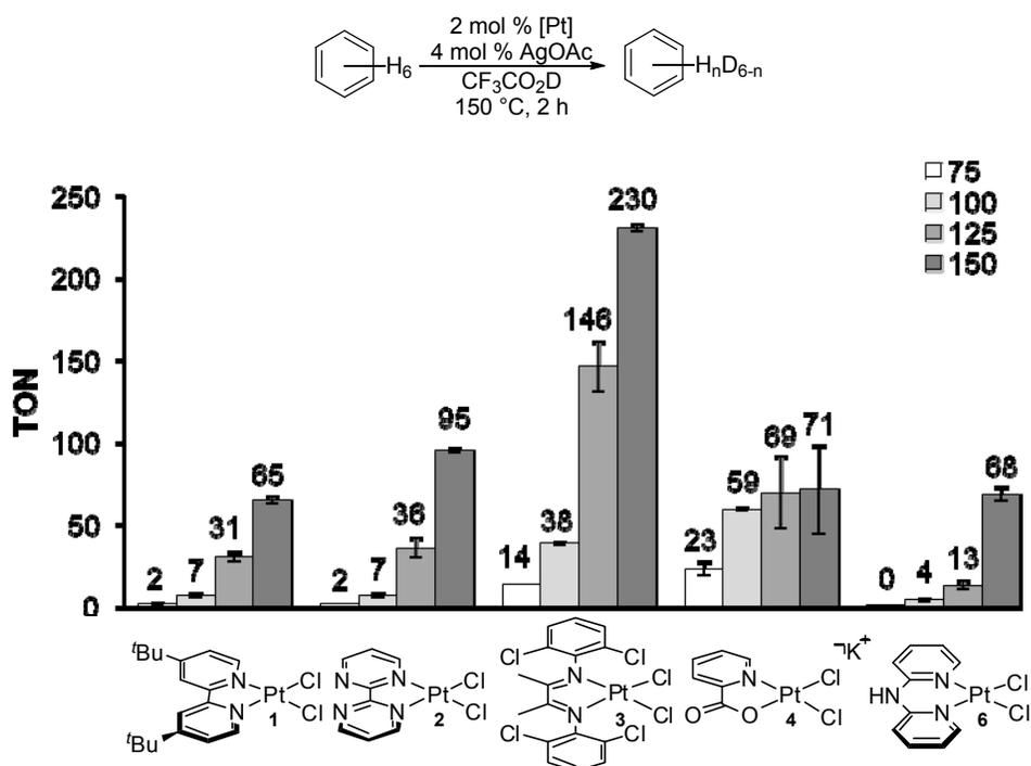
Conditions: Pt<sup>II</sup> catalyst (2 mol %, 5 μmol), benzene (23.2 μL, 0.26 mmol), AgOAc (1.7 mg, 10 μmol) in CF<sub>3</sub>CO<sub>2</sub>D (0.5 mL, 6.5 mmol, 25 equiv relative to benzene) at 150 °C for 2 h. Reported as TON ± standard deviation.
