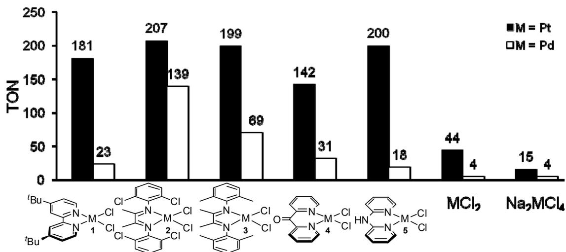
Conditions: M<sup>II</sup> catalyst (2 mol %, 5 μmol), benzene (23.2 μL, 0.26 mmol), AgOAc (2 equiv, 1.7 mg, 10 μmol) in CF<sub>3</sub>CO<sub>2</sub>D (0.5 mL, 6.5 mmol, 25 equiv relative to benzene) at 150 °C for 24 h. Reported as TON.
