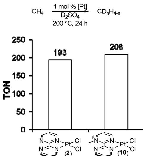
Conditions: Pt<sup>II</sup> catalyst (1 mol %, 20 μmol), CH<sub>4</sub> (~13 bar, 2.0 mmol, 1 equiv), D<sub>2</sub>SO<sub>4</sub> (1 mL, 20 mmol, 10 equiv) at 200 °C for 24 h. Reported TON's are the average of two trials.
