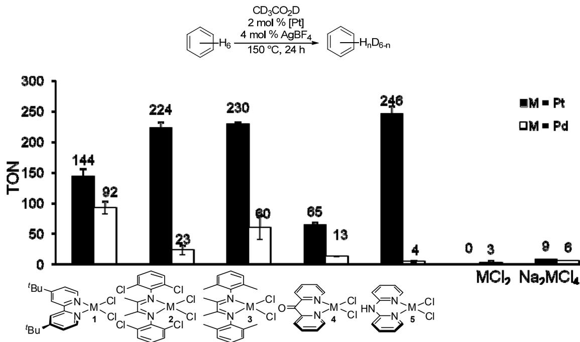
Conditions: Pt<sup>II</sup> catalyst (2 mol %, 5 μmol), benzene (23.2 μL, 0.26 mmol), AgBF<sub>4</sub> (1.9 mg, 10 μmol) in CD<sub>3</sub>CO<sub>2</sub>D (0.37 mL, 6.5 mmol, 25 equiv relative to benzene) at 150 °C.
