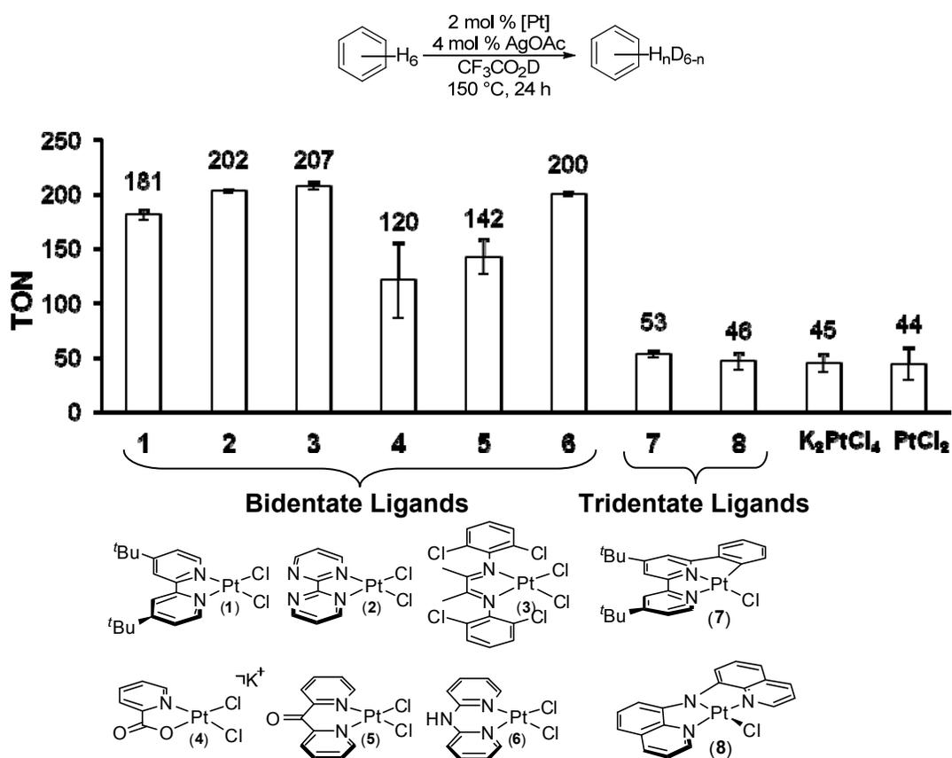
Conditions: Pt<sup>II</sup> catalyst (2 mol %, 5 μmol), benzene (23.2 μL, 0.26 mmol), AgOAc (1.7 mg, 10 μmol) in CF<sub>3</sub>CO<sub>2</sub>D (0.5 mL, 6.5 mmol, 25 equiv relative to benzene) at 150 °C for 2 h and 24 h. Reported as TON ± standard deviation.
