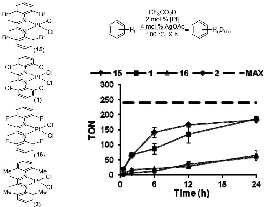
Conditions: Pt<sup>II</sup> catalyst (2 mol %, 5 μmol), benzene (23.2 μL, 0.26 mmol), AgOAc (1.7 mg, 10 μmol) in CF<sub>3</sub>CO<sub>2</sub>D (0.5 mL, 6.5 mmol, 25 equiv relative to benzene) at 100 °C.
