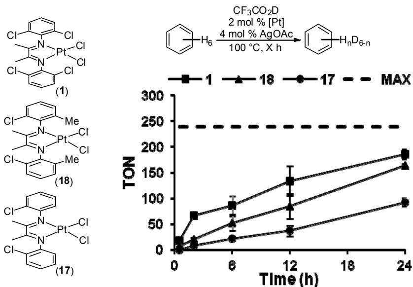
Conditions:  $Pt^{II}$  catalyst (2 mol %, 5  $\mu$ mol), benzene (23.2  $\mu$ L, 0.26 mmol), AgOAc (1.7 mg, 10  $\mu$ mol) in  $CF_3CO_2D$  (0.5 mL, 6.5 mmol, 25 equiv relative to benzene) at 100 °C.
