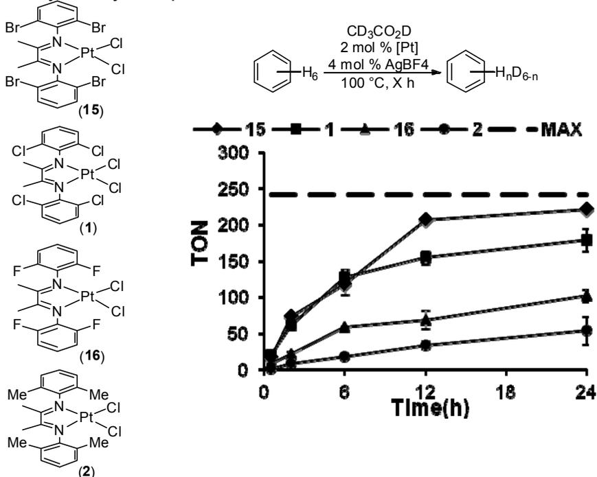
Conditions: Pt<sup>II</sup> catalyst (2 mol %, 5 μmol), benzene (23.2 μL, 0.26 mmol), AgBF<sub>4</sub> (1.9 mg, 10 μmol) in CD<sub>3</sub>CO<sub>2</sub>D (0.37 mL, 6.5 mmol, 25 equiv relative to benzene) at 100 °C.
