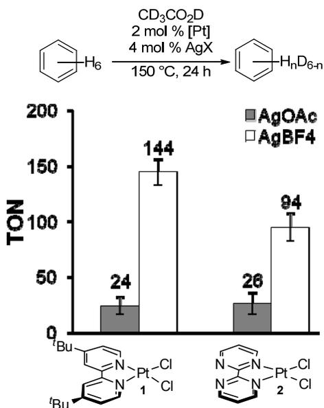
Conditions: Pt<sup>II</sup> catalyst (2 mol %, 5 μmol), benzene (23.2 μL, 0.26 mmol), AgOAc (1.7 mg, 10 μmol) or AgBF<sub>4</sub> (1.9 mg, 10 μmol) in CD<sub>3</sub>CO<sub>2</sub>D (0.37 mL, 6.5 mmol, 25 equiv relative to benzene) at 150 °C for 24 h. Reported as TON ± standard deviation.
