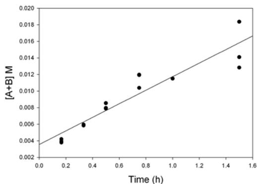
Conditions: Catalyst **5b** (2.0 mg, 3.68  $\mu\text{mol}$ , 5 mol %), naphthalene- $d_8$  (50.1 mg, 0.368 mmol, 5 equiv),  $[\text{Ph}_2]\text{BF}_4$  (27.1 mg, 0.0735 mmol, 1 equiv) in nitrobenzene (0.75 mL). Yield and selectivity were determined by GC analysis. The data was plotted using Sigma Plot 10 and fit to the function  $f=y_0+a*x$ ;  $a = 8.2*10^{-3} \pm 0.8*10^{-3}$ ,  $y_0 = 3.6*10^{-3} \pm 0.7*10^{-3}$ ,  $R^2 = 0.8752$ .
