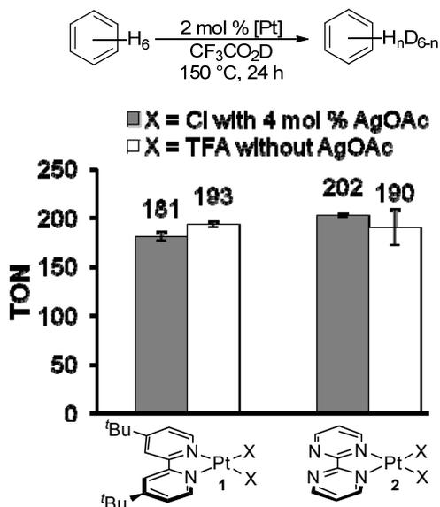
Conditions: Pt<sup>II</sup> catalyst (2 mol %, 5 μmol), benzene (23.2 μL, 0.26 mmol), AgOAc (2 equiv, 1.7 mg, 10 μmol) in CF<sub>3</sub>CO<sub>2</sub>D (0.5 mL, 6.5 mmol, 25 equiv relative to benzene) at 150 °C for 24 h. Reported as TON ± standard deviation.
