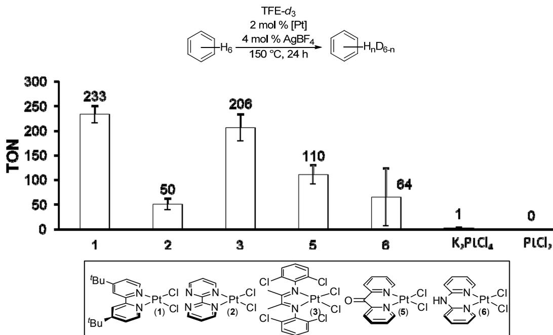
Conditions: Pt<sup>II</sup> catalyst (2 mol %, 5 μmol), benzene (23.2 μL, 0.26 mmol), AgBF<sub>4</sub> (1.9 mg, 10 μmol) in TFE-*d*<sub>3</sub> (0.47 mL, 6.5 mmol, 25 equiv relative to benzene) at 150 °C for 24 h. Reported as TON ± standard deviation.
