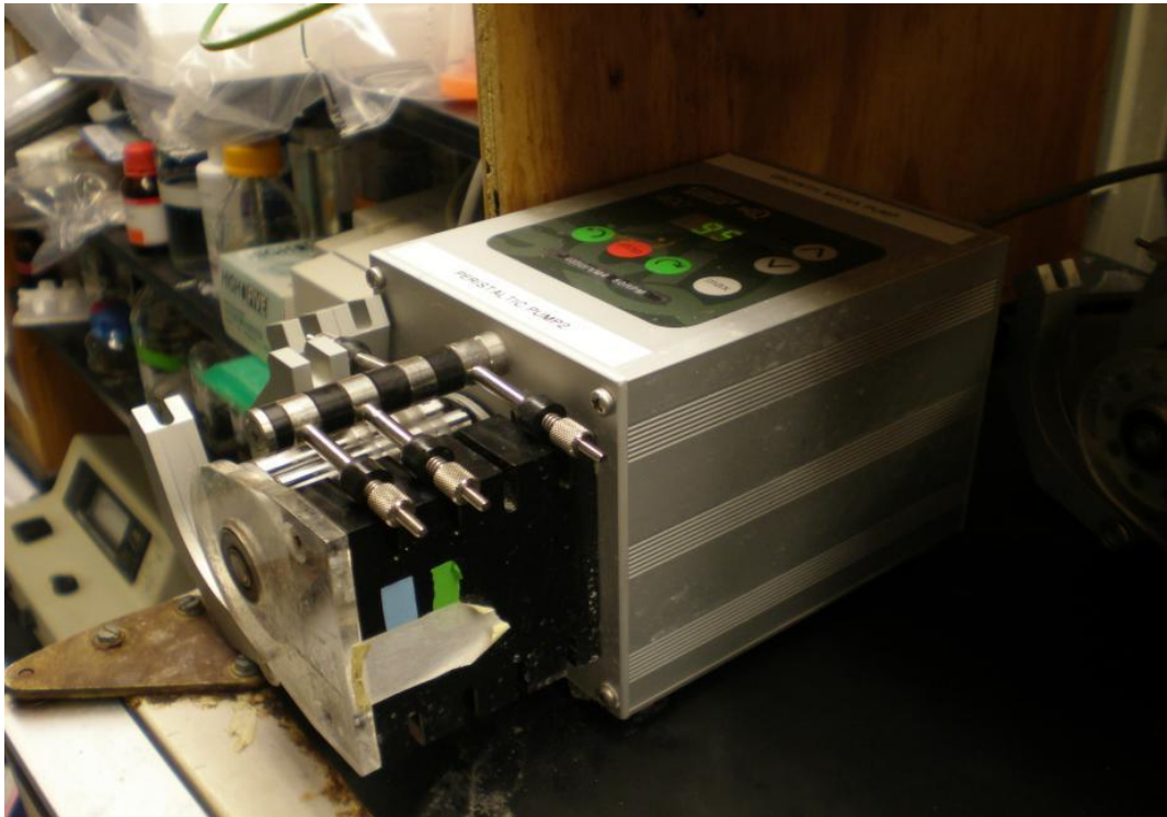
Figure 2-1 Alitea VS series peristaltic pump This kind of pump was used to pump media into and out from the culture, and to take a sample of the system every ½ hour. This pump can be controlled from a computer via a serial port.
