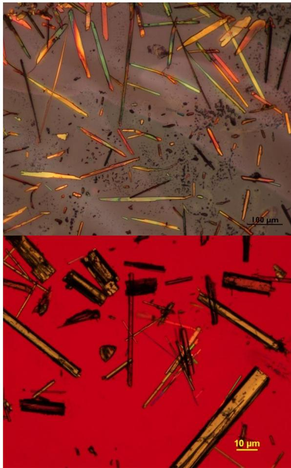
Figure 3.4. Transmitted light optical micrograph of DCHD single crystals (little amount of cracks developed along the [001] (chain) direction)
