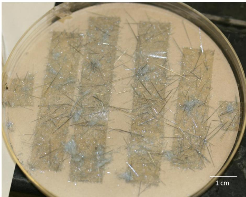
Figure 3.3. Single crystals of DCHD diacetylene grown at room temperature.
