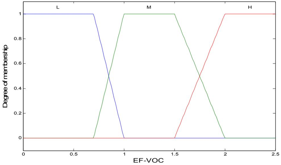
**Figure 6.12: Membership Functions for the Fuzzy Input Variable EF-VOC**
