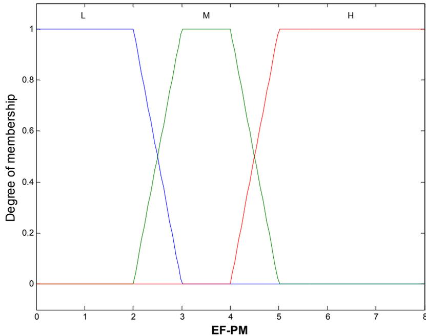
**Figure 6.3: Membership Functions for the Fuzzy Input Variable Emission Factors of PM (EF-PM)**
