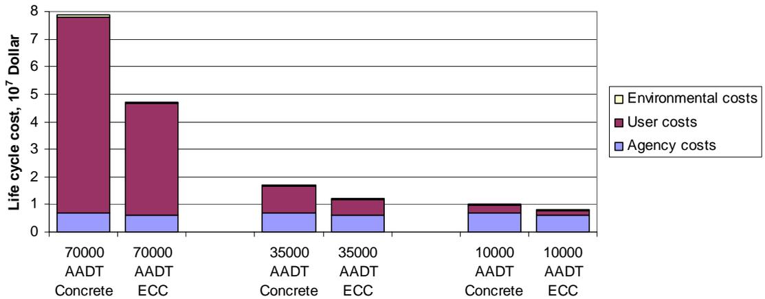
**Figure A.2 Total life cycle cost of different AADT cases for concrete and ECC overlay systems**
