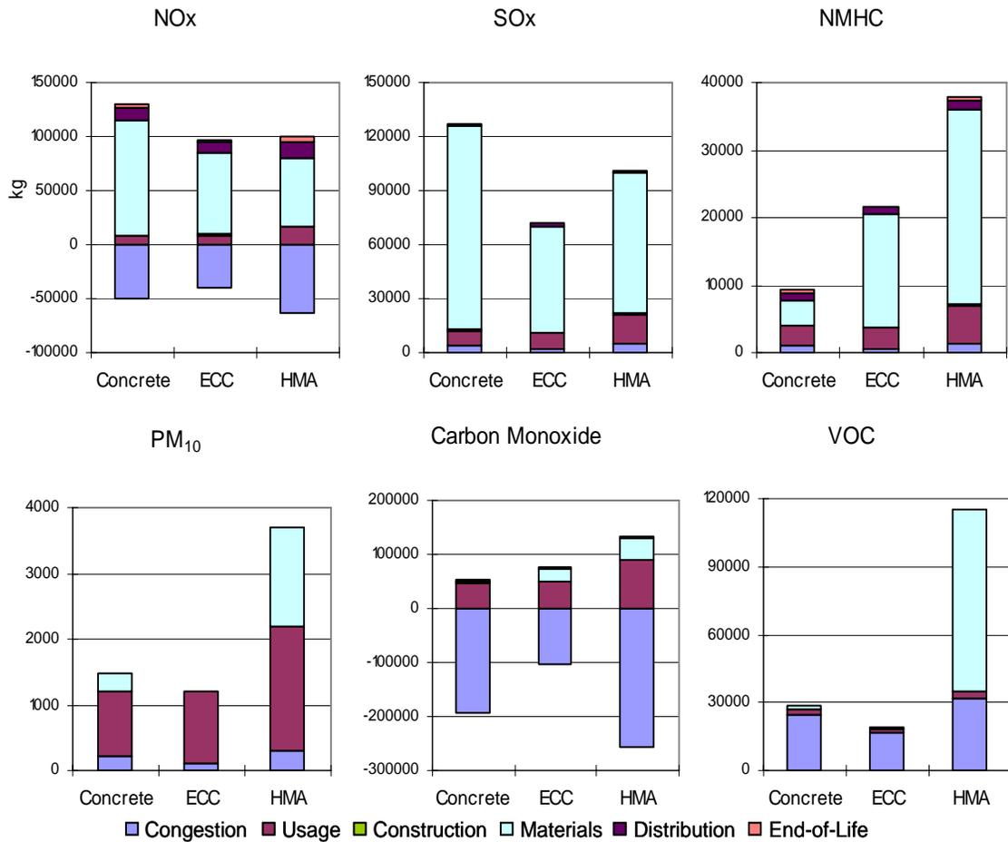
**Figure 2.9 Air emissions by life cycle phase**
