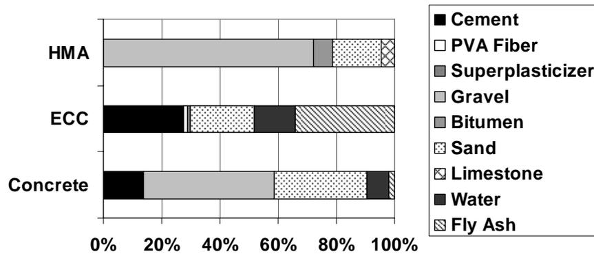
**Figure 2.4 Material composition of concrete, HMA, and ECC materials**
