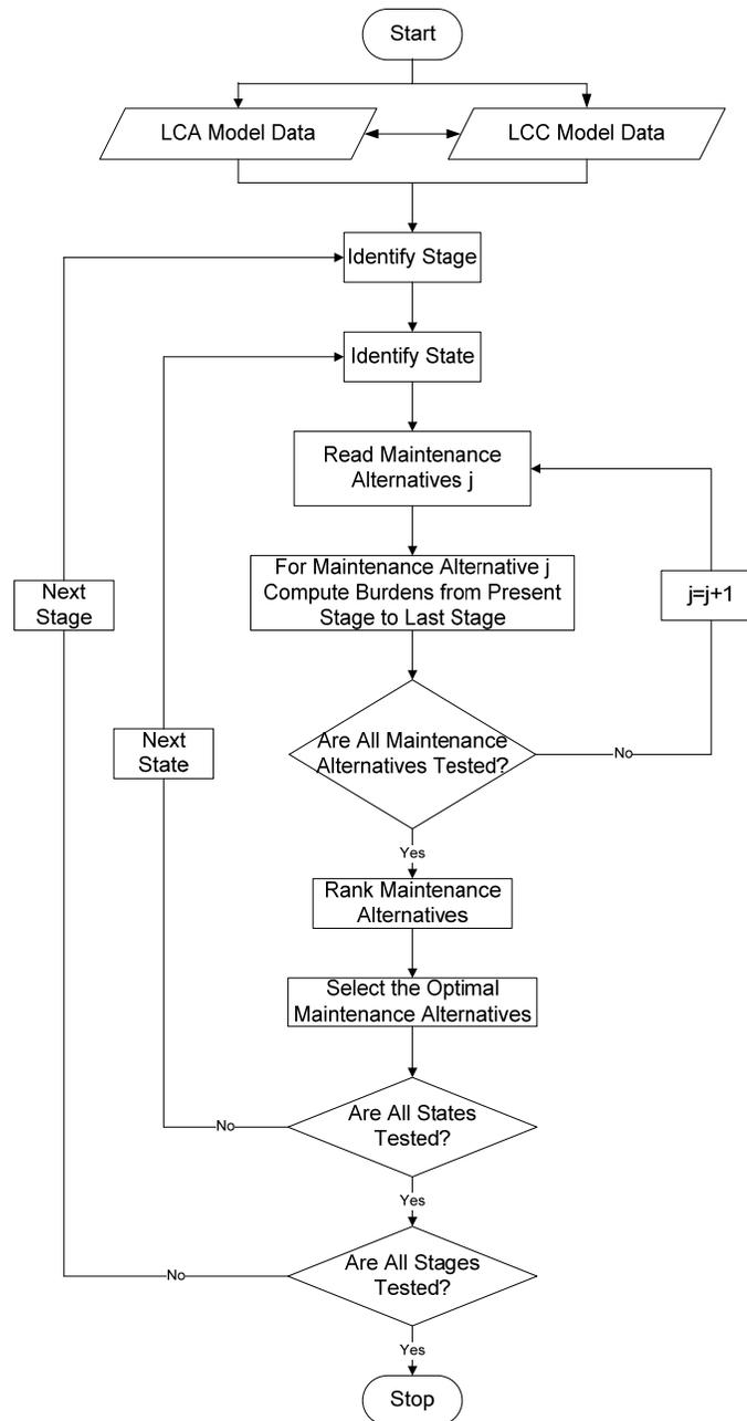
**Figure 3.1 LCO model operation flowchart using dynamic programming**
