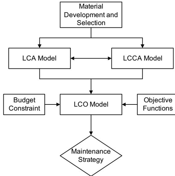
**Figure 4.2 The process of project-level pavement asset management system**
