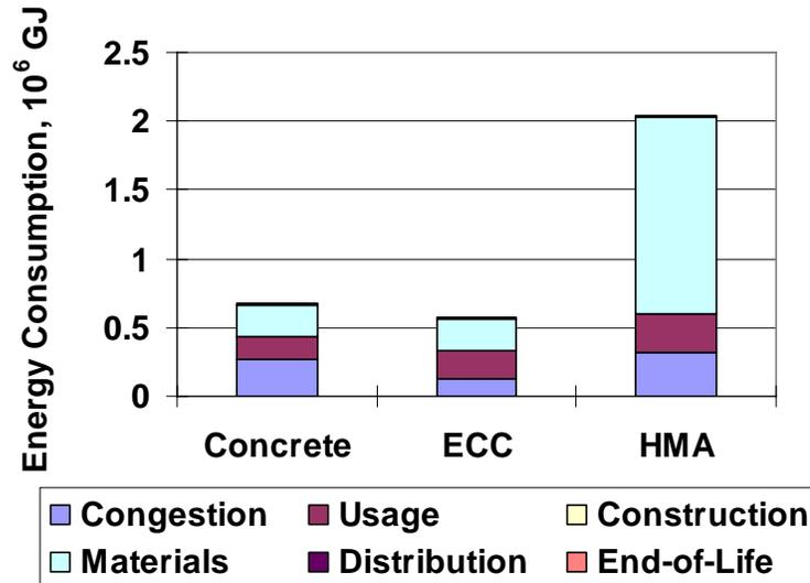
Figure 2.7 Life cycle energy consumption by life cycle phase
