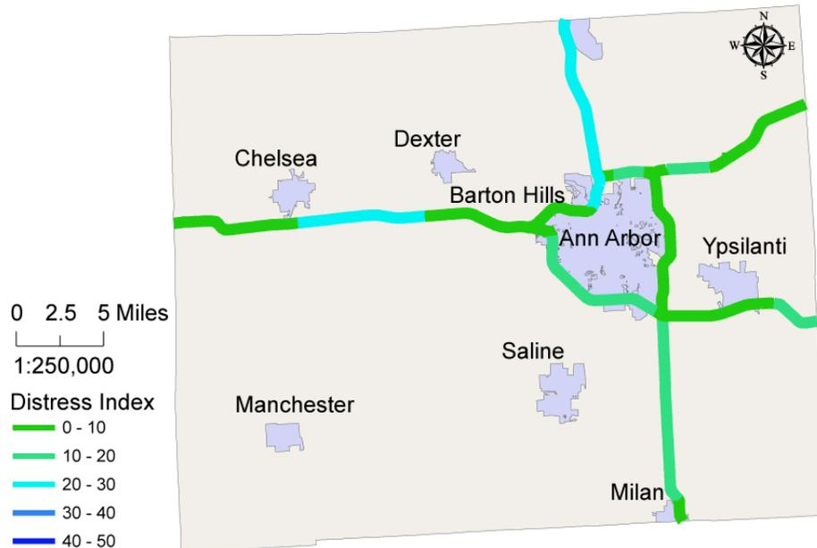
**Figure 5.4 GIS map and pavement network condition**
