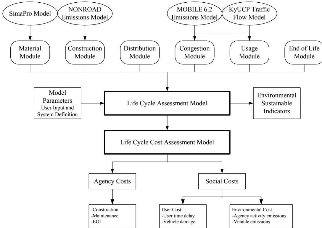
**Figure 2.3 Integrated LCA-LCCA model framework**
