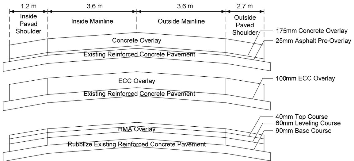
**Figure 2.1 Overlay structure and thickness in one direction**
