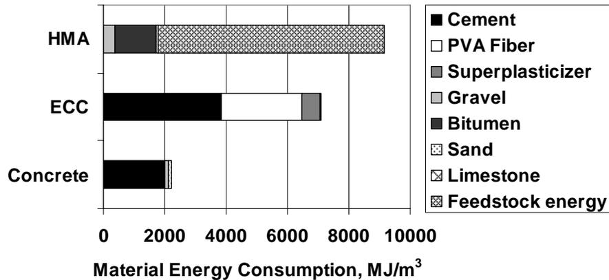
**Figure 2.5 Primary energy consumption per volume of each material**
