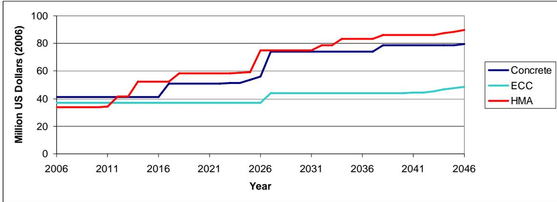
**Figure 2.11 Cumulative life cycle costs for overlay systems**
