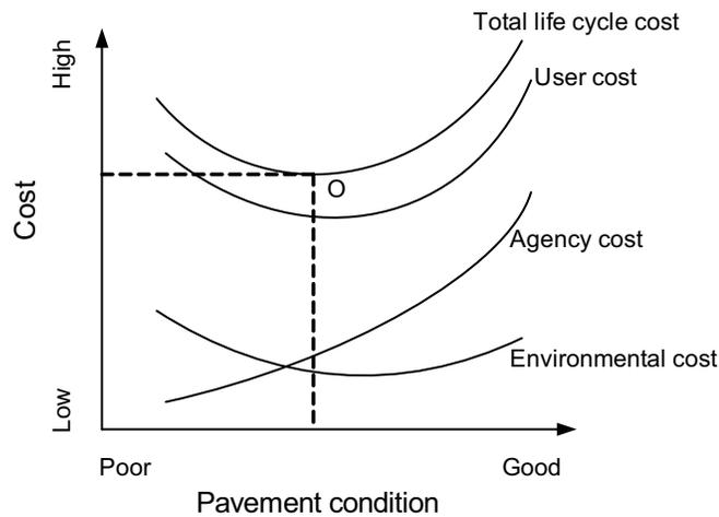
**Figure 4.3 A hypothetical relationship between pavement condition and cost**
