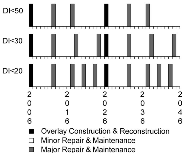
**Figure B.1 Optimal preservation strategies for an HMA overlay system based on different pavement condition constraints**
