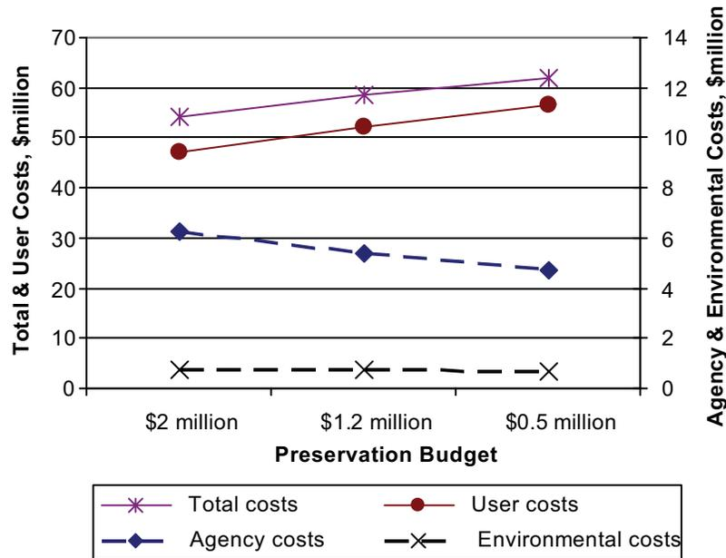
**Figure 4.6 Total life cycle cost based on different budget constraints for a 20 year analysis period**
