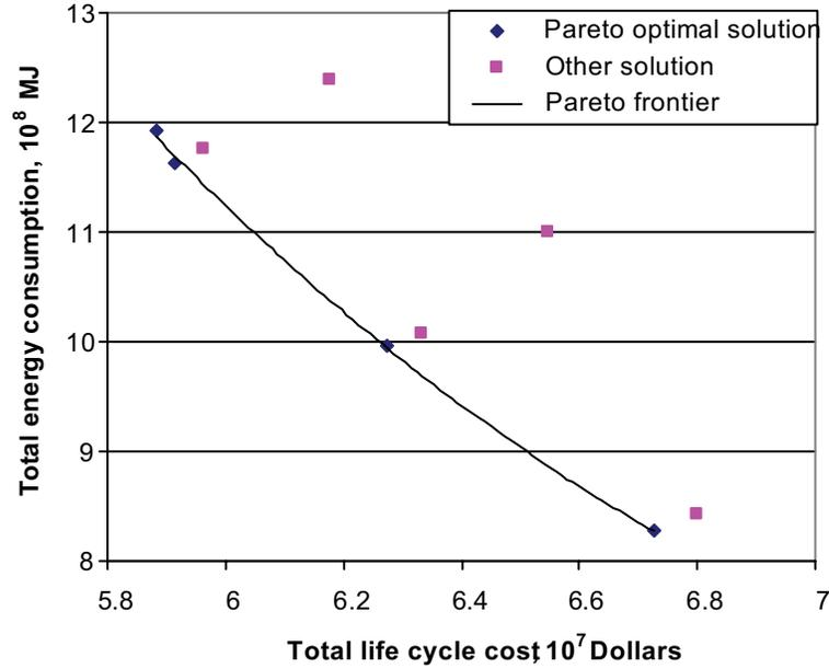
**Figure 4.7 Pareto frontier for total energy consumption and total life cycle cost objectives for a 20 year analysis period**
