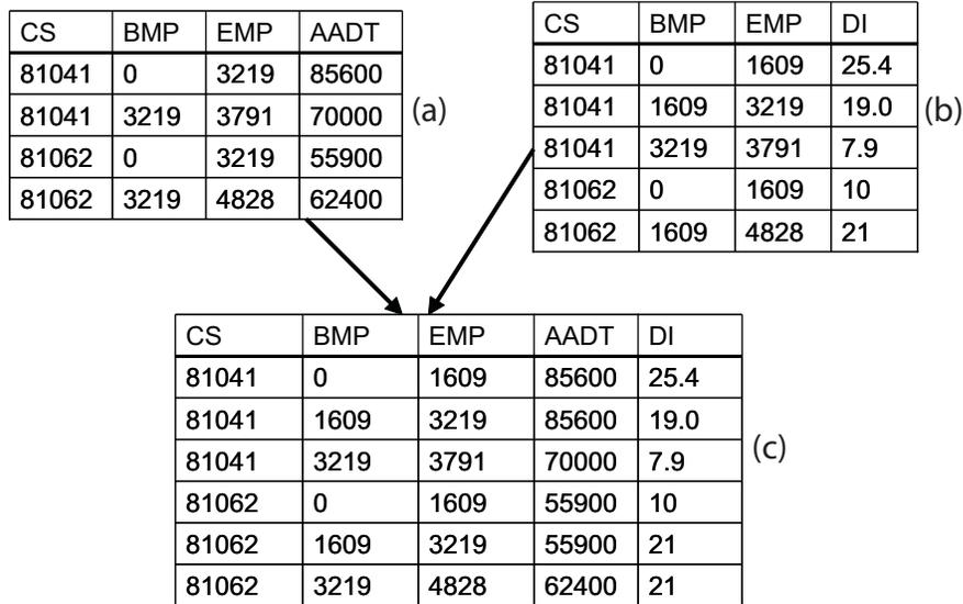
**Figure 5.3 Union of two route event tables using dynamic segmentation**
