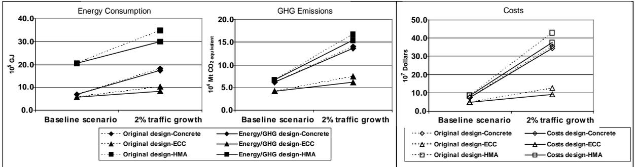
Figure 3.5 Life cycle results with different annual traffic growth rate
