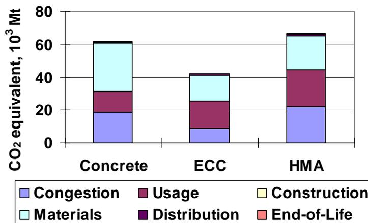
Figure 2.8 Greenhouse gas emissions by life cycle phase
