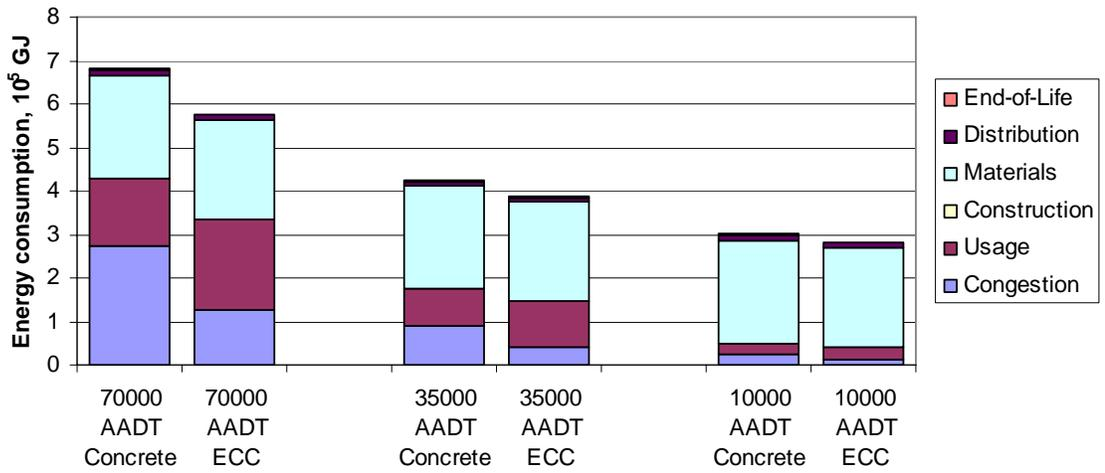
**Figure A.1 Total life cycle energy consumption of different AADT cases for concrete and ECC overlay systems**
