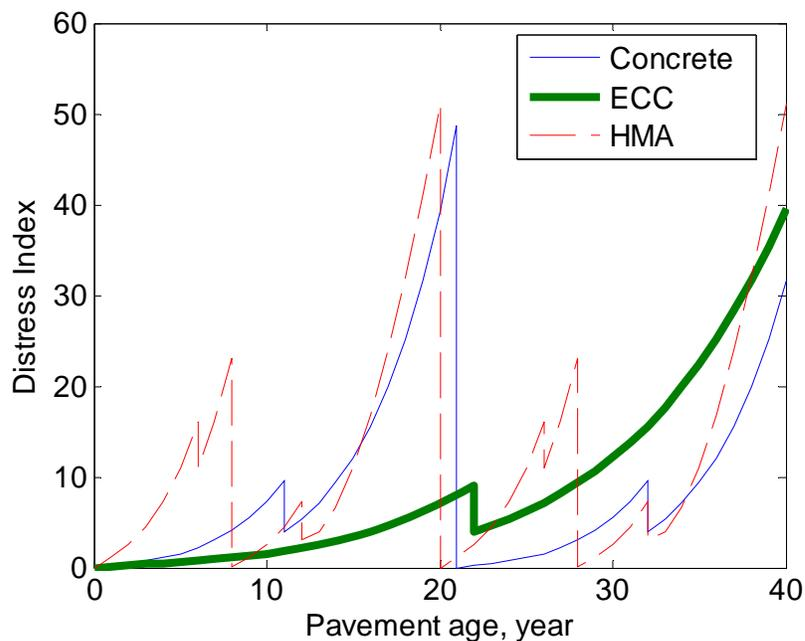
**Figure 2.6 Distress index of each pavement**
