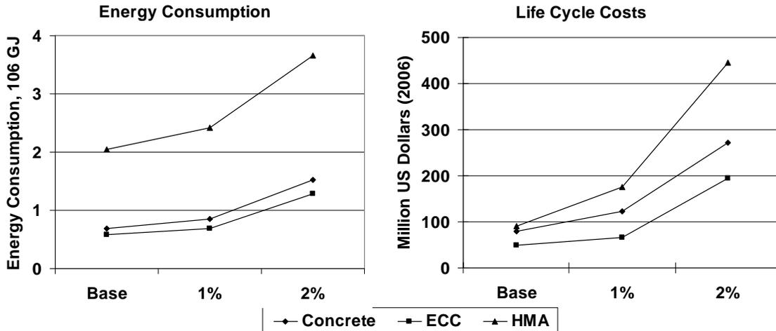
**Figure 2.12 Energy consumption and life cycle costs at different traffic growth rate**
