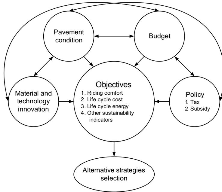
**Figure 4.1 Pavement asset management system framework**
