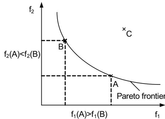
**Figure 4.4 Multi-objective optimization and Pareto efficiency**
