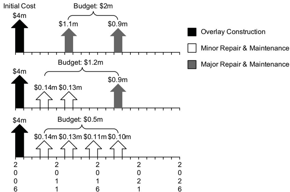
**Figure 4.5 Optimal maintenance strategies based on different budget constraints**
