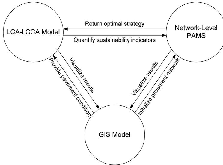
**Figure 5.1 The integrated framework of the network-level PAMS**
