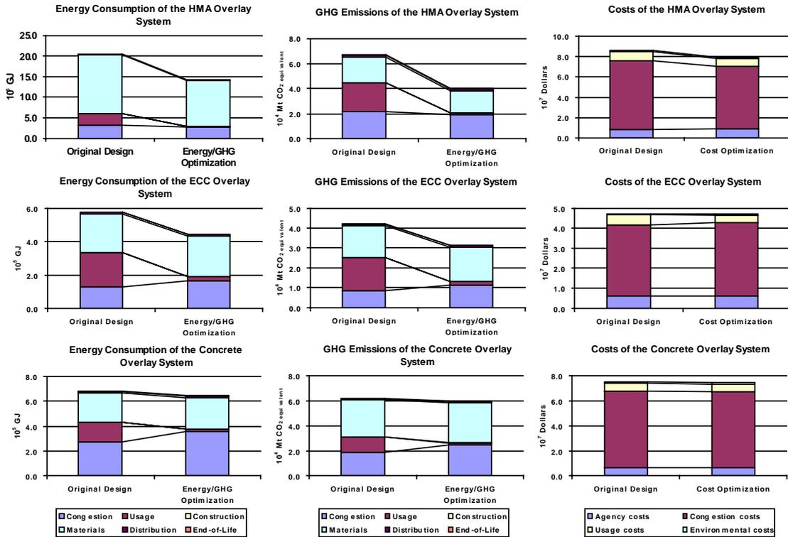
**Figure 3.3 Comparison of energy consumption, GHG emissions and costs for MDOT preservation strategies and optimal strategies for a. HMA, b. ECC, and c. Concrete overlay systems**
