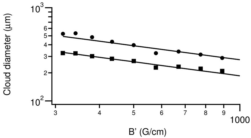
Figure 4.10: MOT cloud rms diameter vs.  $B'$ . Parameters are:  $P = 0.8$  mW,  $\delta = -0.6$ , and  $w = 2.5$  mm. A characterization is provided by the longest (circles) and shortest (squares) rms size of the elliptical MOT. The diameter is about 5 times larger than what Doppler theory predicts. The solid lines show the  $(B')^{-1/2}$  dependence expected from eqn. 4.16.
