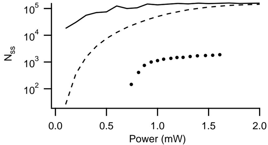
Figure 4.12: Observed steady-state atom number vs. power. Experimental observations (points) for  $\delta = -0.7$ ,  $B' = 500$  G/cm and  $w = 2.5$  mm are shown with the 1-D (solid line) and 3-D (dotted line) models.
