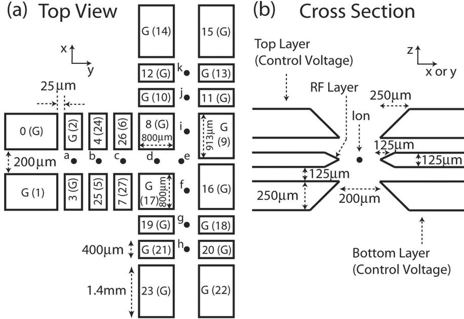
Figure 3.1: Top view and cross-section of two-dimensional “T” trap array. Dots depict the location of trapping zones, labelled a-k. The outer control electrodes are labelled 0-27, with bottom layer electrodes in parentheses. Electrodes labeled by G are internally grounded.
