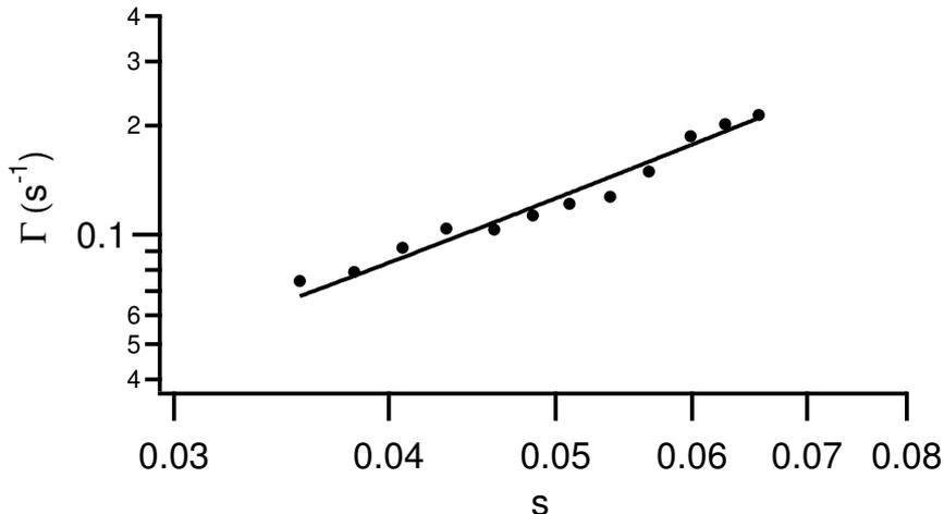
Figure 4.7: Observed MOT loading rate vs. saturation parameter  $s = I/I_{sat}$ . The power is varied for a constant beam waist of  $w = 1.25$  mm. The photoionization cross section out of the  $^1P_1$  state is determined from a quadratic fit to  $s$  given by eqn. 4.3. Extrapolating the curve to zero intensity (not shown here) gives information on the loss rate due to collisions with background gas.
