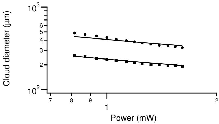
Figure 4.13: MOT cloud diameter vs. total MOT laser power. Parameters are:  $\delta = -0.6$ ,  $B' = 500$  G/cm and  $w = 2.5$  mm. The solid lines show the expected dependence of the MOT diameter on power from eqn. 4.16.
