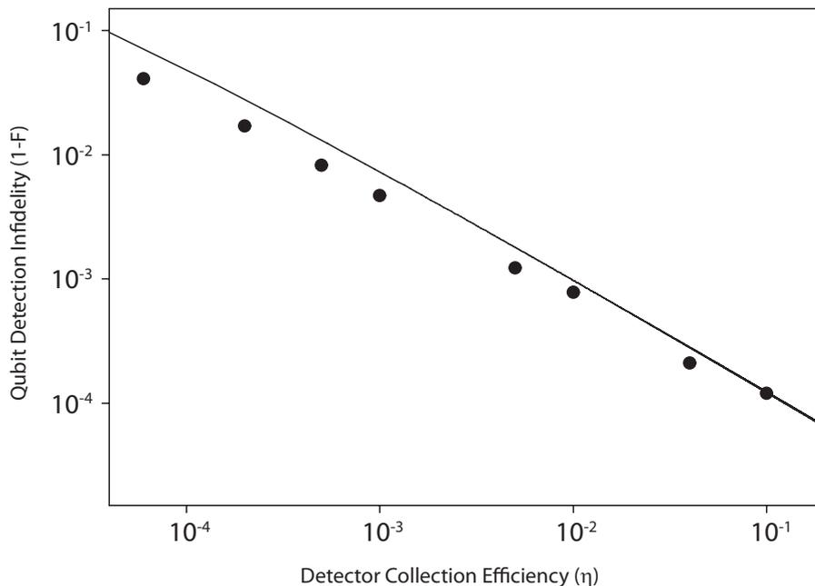
Figure 2.5: Theoretical prediction of detection infidelity (1-F) using the  $P_{3/2}$  detection scheme for  $^{111}\text{Cd}^+$  as a function of total detector collection efficiency ( $\eta$ ). Filled circles are numerically calculated using eqn. 2.17 with iterations to find the optimal light level and detection time for each  $\eta$ ; solid curve uses the approximate analytic result of eqn. 2.19.
