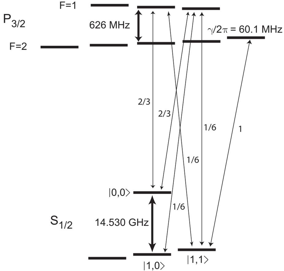
Figure 2.3: Relevant energy levels and relative dipole transition strengths for state detection of  $^{111}\text{Cd}^+$ . Note that the Zeeman splitting ( $< 10$  MHz) is small compared to the hyperfine splittings.
