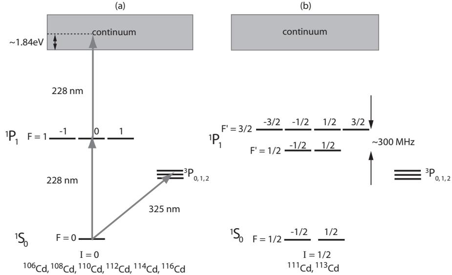
Figure 4.1: Neutral Cd energy level diagram. a) The bosonic (even) isotopes ( $I=0$ ) of Cd. b) The fermionic (odd) isotopes ( $I=1/2$ ) of Cd, where the  $^1P_1$  hyperfine splitting arises from  $(\mathbf{L} \cdot \mathbf{I})$  coupling. Individual levels are labeled with  $m_F$ . Note that diagram is not to scale.
