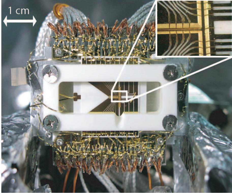
Figure 3.2: Photograph of T-junction trap array. The magnified inset shows the trapping array near the junction.
