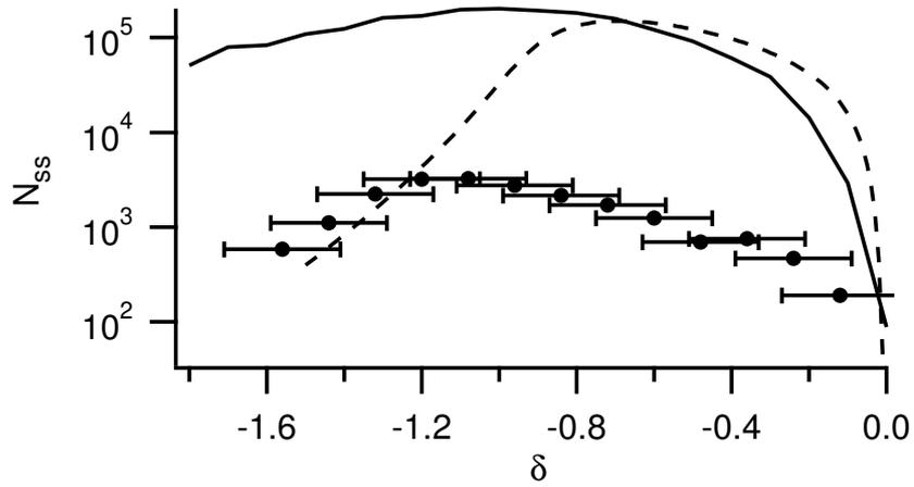
Figure 4.11: Observed steady-state atom number vs. detuning ( $\delta$ ). Experimental observations (points) along with the 1-D (dotted line) and 3-D (solid line) models are shown for  $P = 1.8$  mW,  $B' = 500$  G/cm and  $w = 2.5$  mm.
