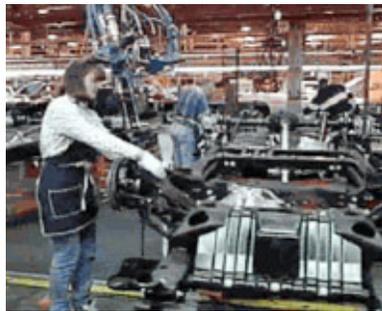
Figure 1.4: Chassis Assembly (Courtesy: General Motors Corporation, 2008d)
