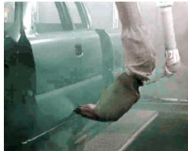
Figure 1.3: Primer coat application (Courtesy: General Motors Corporation, 2008c)
