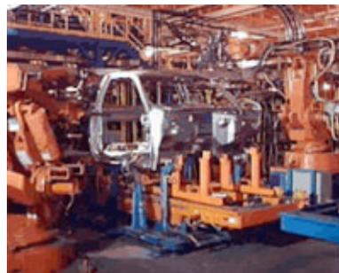
Figure 1.2: Assembly of truck cab (Courtesy: General Motors Corporation, 2008b)
