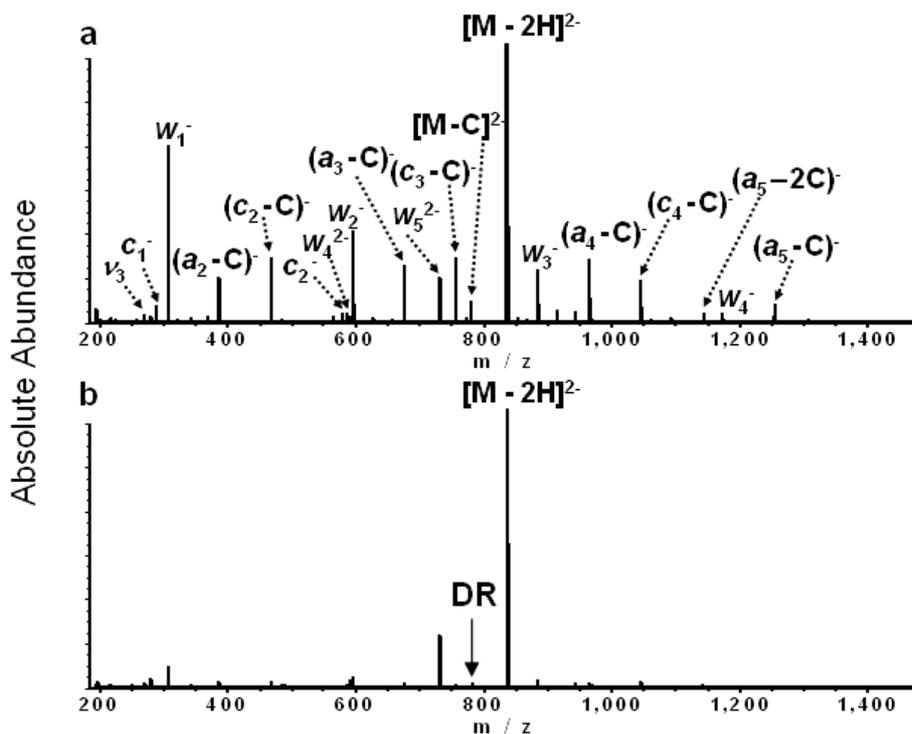
Figure 5-2. IRMPD spectra of doubly deprotonated  $dC_6$  without (a) and with (b) DR ejection at the ICR frequency of  $[M - C]^{2-}$ . (The solid arrow indicates the  $m/z$  corresponding to the frequency of the DR rf waveform).
