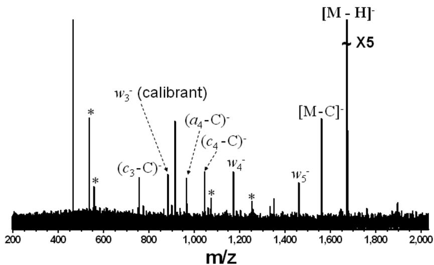
Figure B-3. EID (18.1 eV electrons, 2 s, 32 scans) of singly deprotonated  $dC_6$ .  $d/w$ ,  $(a/z - B)$ ,  $(d/w - B)$ , and  $(c/x - B)$  ions are observed. Electronic noise spikes are labeled with asterisks.
