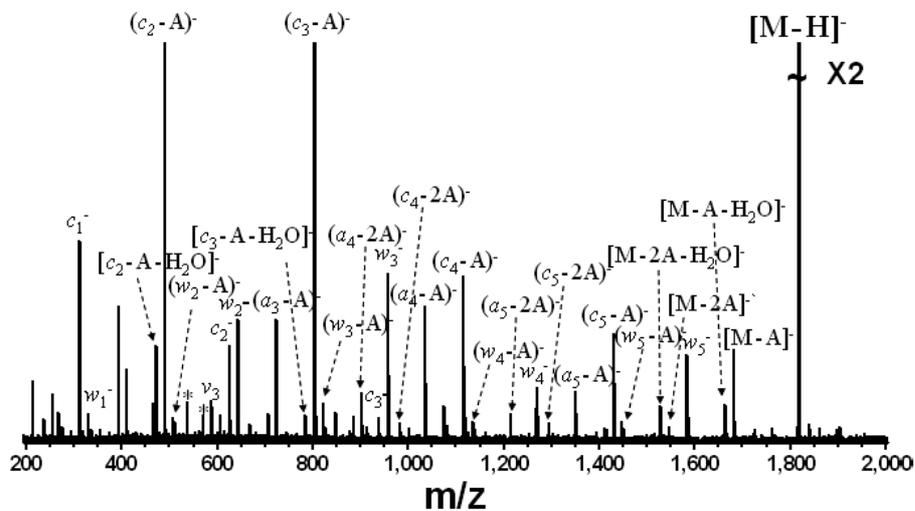
Figure B-2. IRMPD (10 W, 20 ms, 32 scans) of singly deprotonated  $dA_6$ . Mainly  $c/x$ ,  $d/w$ ,  $(a/z - B)$ ,  $(d/w - B)$  and  $(c/x - B)$  ions are observed. Electronic noise spikes are labeled with asterisks.
