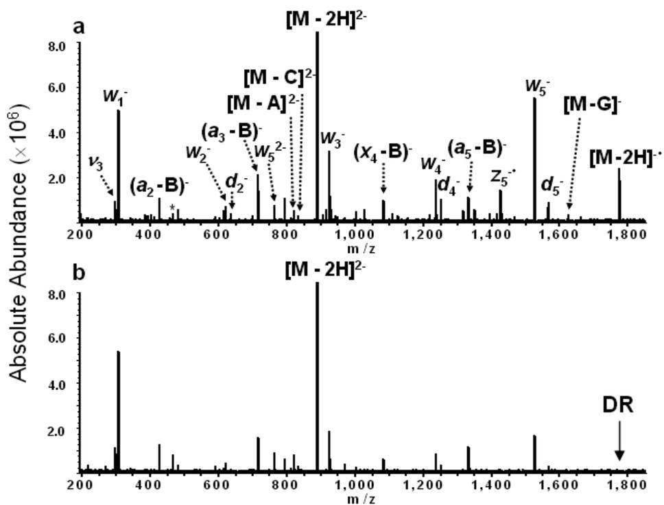
Figure 5-8. EDD spectra of doubly deprotonated d(GCATAC) without DR (a) and with DR ejection at the frequency of  $[M - 2H]^-$  (b). (the solid arrow indicates the  $m/z$  value corresponding to the frequency of the DR rf waveform, \* = electronic noise spike).
