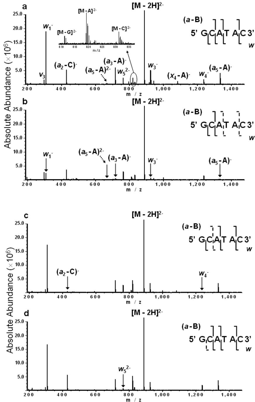
Figure 5-4. IRMPD spectra of doubly deprotonated d(GCATAC) without DR (a) and with DR ejection at the ICR frequencies of  $[M - A]^{2-}$  (b),  $[M - C]^{2-}$  (c), and  $[M - G]^{2-}$  (d). (solid arrows indicate product ions that were significantly decreased in abundance).
