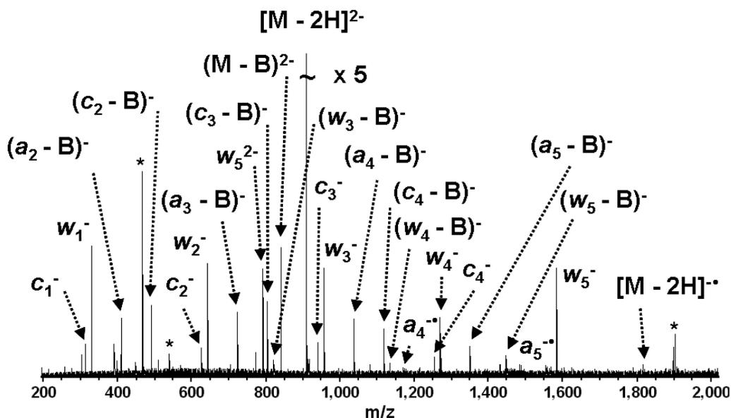
Figure 2-5. EDD (17 eV electrons, 1 s irradiation, 30 scans) of  $dA_6$  with an indirectly heated hollow dispenser cathode electron source. Much more extensive fragmentation is observed compared to the filament EDD shown in Figure 2-4. Only one label is given for  $d/w$ ,  $c/x$  and  $a/z$  ion series. Increases in fragmentation efficiency and sensitivity are also evident. Electronic noise spikes are labeled with asterisks.
