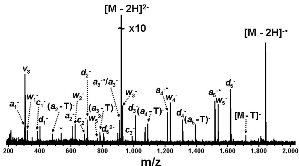
Figure 2-9. EDD of  $\text{pdT}_6$  (2 s irradiation, - 18.1 V bias, 32 scans) results in complete  $d$  and  $w$  ion series. For  $a^\bullet$  ions, complementary to the  $w$  ions, radical-mediated nucleobase loss is observed. Electronic noise spikes are labeled with asterisks.
