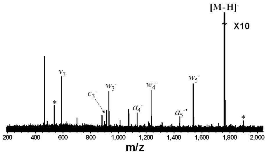
Figure B-5. EID (18.1 eV electrons, 2 s, 32 scans) of singly deprotonated  $dT_6$ . Mainly  $d/w$ ,  $c/x$ , and  $b/y$  ions are observed. Electronic noise spikes are labeled with asterisks.
