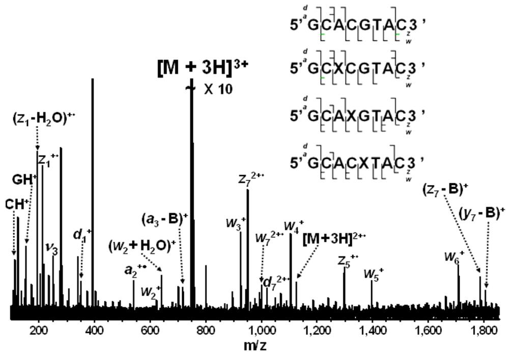
Figure 6-19. ECD (- 1 V bias voltage, 15 ms, 88 scans) of triply protonated d(GCACXTAC) (X denotes an abasic site at which a nucleobase has been replaced by hydrogen). The inset summarizes observed backbone ECD bond cleavages for this oligonucleotide and three related ones for which X is at a different position.
