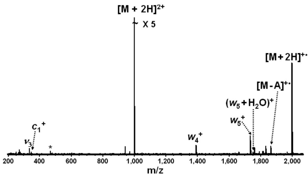
Figure 6-2. ECD (-1 V bias voltage, 45 ms, 50 scans) of doubly protonated 2'-methoxy  $A_6$ . Product ions labeled  $w$  can also be  $d$  ions, and the ion labeled  $c$  can also be an  $x$  ion. Abundant charge reduced precursor ions are observed. Electronic noise spike is labeled with an asterisk.
