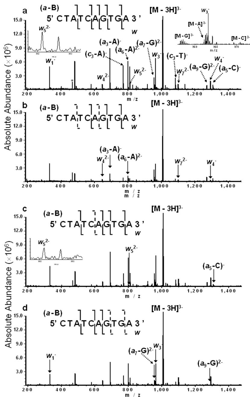
Figure 5-6. IRMPD spectra of triply deprotonated d(CTATCAGTGA) without DR (a) and with DR ejection at the ICR frequencies of [M - A]<sup>3-</sup> (b), [M - C]<sup>3-</sup> (c), and [M - G]<sup>3-</sup> (d). (solid arrows indicate product ions that were significantly decreased, \* = electronic noise spikes).
