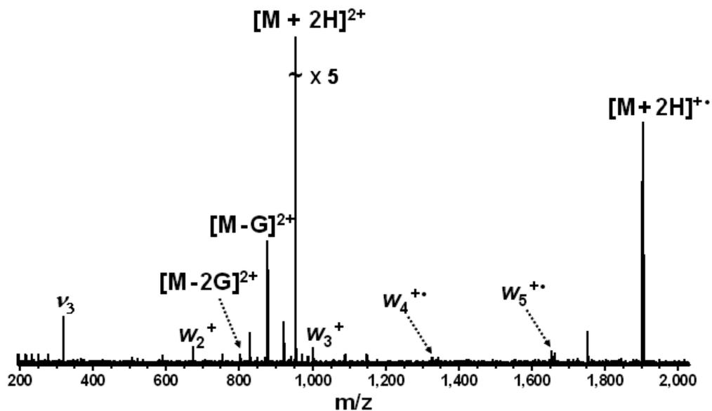
Figure 6-12. ECD (- 1 V bias voltage, 30 ms, 32 scans) of doubly protonated methylphosphonate-containing dG<sub>6</sub>. *d/w* ions are labeled as *w* ions.
