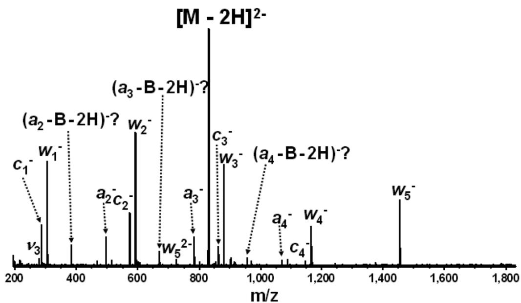
Figure 6-14. EDD of doubly deprotonated methylphosphonate-containing dC<sub>6</sub>. Product ions labeled *w* can also be *d* ions, ions labeled *a* can also be *z* ions, and ions labeled *c* can also be *x* ions. A complete series of *d/w* ions is observed, allowing full sequencing of the oligonucleotide. Question marks denote assignments with high (>20 ppm) mass error.
