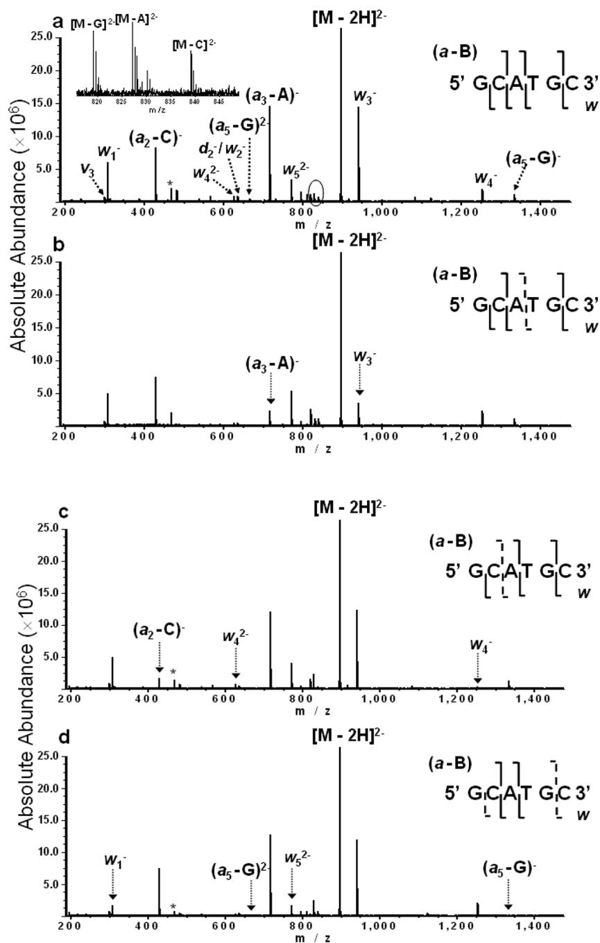
Figure 5-5. IRMPD spectra of doubly deprotonated d(GCATGC) without DR (a) and with DR ejection at the ICR frequencies of  $[M - A]^{2-}$  (b),  $[M - C]^{2-}$  (c), and  $[M - G]^{2-}$  (d). (solid arrows indicate product ions that were significantly decreased in abundance, \* = electronic noise spikes).
