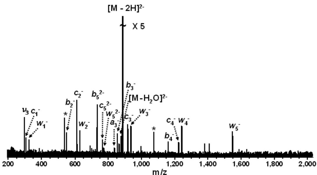
Figure 4-9. EDD (- 18.1 V bias voltage, 2 s irradiation, 32 scans) of the RNA U<sub>6</sub>. A complete *d/w* ion series is observed, allowing full sequencing of the oligonucleotide. Electronic noise spikes are labeled with asterisks.
