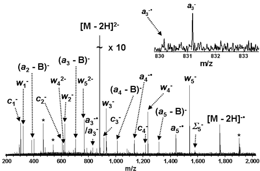
Figure 2-8. EDD (17 eV electrons, 1 s irradiation, 20 scans) of  $dT_6$  with an indirectly heated hollow dispenser cathode electron source. The data is similar to EDD of  $dA_6$ ,  $dC_6$ , and  $dG_6$ . The inset illustrates the mixture of radical and even-electron species for the  $a_3/z_3$  ion. Only one label is given for *d/w*, *c/x* and *a/z* ion series. Electronic noise spikes are labeled with asterisks.
