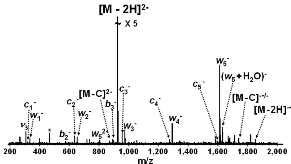
Figure 6-5. EDD (-18.2 V, 2 s, 50 scans) of doubly deprotonated 2'-methoxy C<sub>6</sub>. Product ions labeled  $w$  can also be  $d$  ions, ions labeled  $b$  can also be  $y$  ions, and ions labeled  $c$  can also be  $x$  ions. Full series of  $c/x$  and  $d/w$  ions are observed, allowing full sequencing of the oligonucleotide. Electronic noise spike is labeled with an asterisk.
