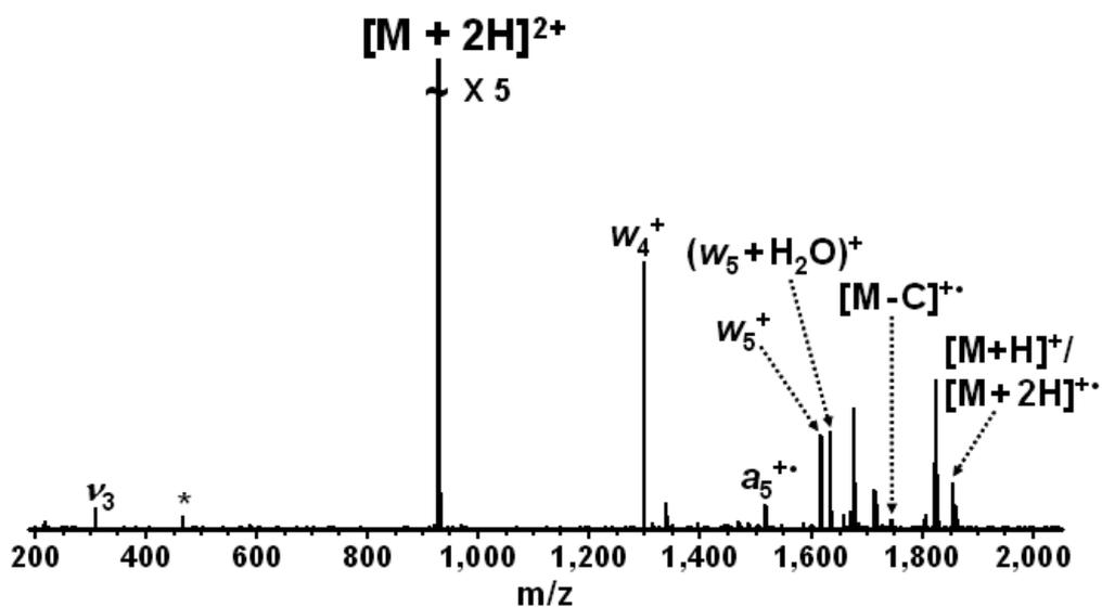
Figure 6-1. ECD (-1 V bias voltage, 40 ms, 50 scans) of doubly protonated 2'-methoxy C<sub>6</sub>. Product ions labeled *w* can also be *d* ions, and the ion labeled *a* can also be a *z* ion. Electronic noise spike is labeled with an asterisk.
