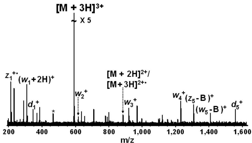
Figure 6-13. ECD (- 1 V bias voltage, 30 ms, 32 scans) of triply protonated methylphosphonate-containing d(GCATAC). Full sequence coverage is obtained from the combination of *w* and *d* ion series.
