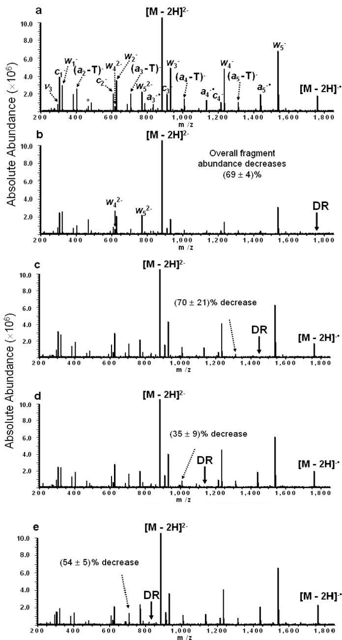
Figure 5-7. EDD spectra of doubly deprotonated  $dT_6$  without DR (a) and with DR ejection at the frequencies of  $[M-2H]^\bullet$  (b),  $a_5^\bullet$  (c),  $a_4^\bullet$  (d), and  $a_3^\bullet$  (e). (solid arrows indicate  $m/z$  values corresponding to the frequencies of the DR rf waveforms, \* = electronic noise spikes). Ions labeled  $w$  can also be  $d$  ions, ions labeled  $a$  can also be  $z$  ions, and ions labeled  $c$  can also be  $x$  ions.
