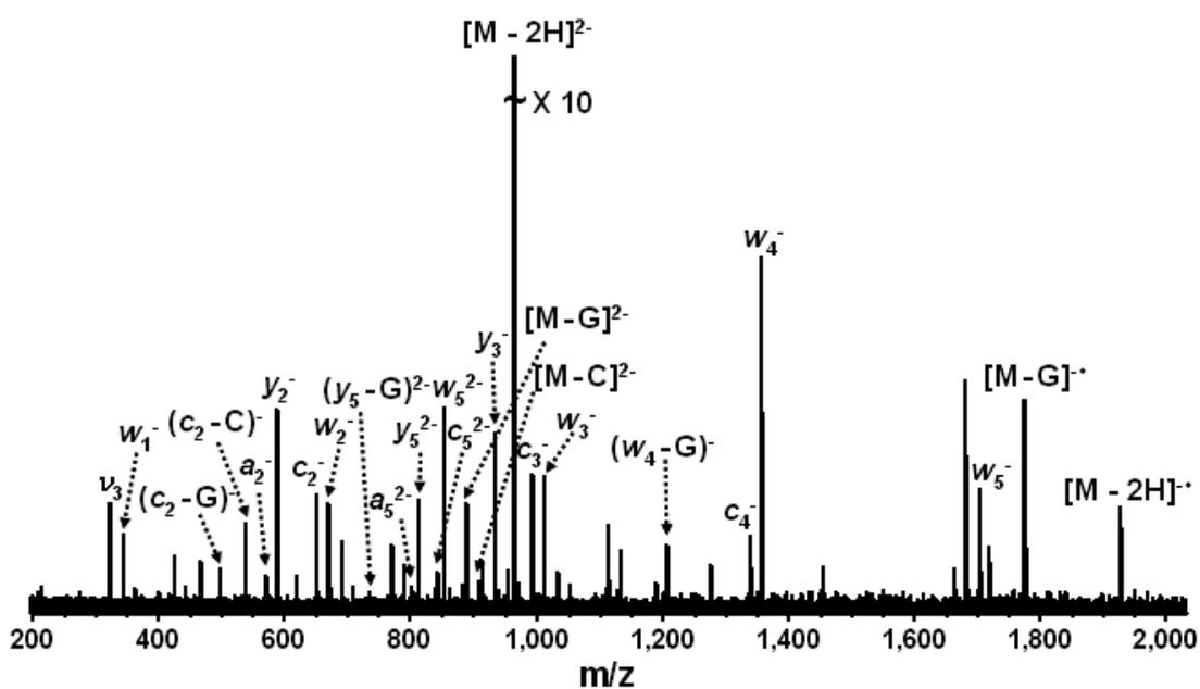
Figure 4-8. EDD (- 18.2 V bias voltage, 2 s irradiation, 32 scans) of the RNA CGGGGC. Again, complete *d/w* and *c/x* ion series are observed, allowing full sequencing of the oligonucleotide. Electronic noise spikes are labeled with asterisks.
