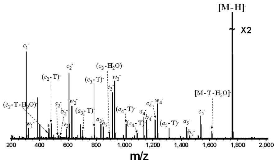
Figure B-6. IRMPD (10 W, 20 ms, 32 scans) of singly deprotonated  $\text{dT}_6^-$ . Mainly  $a/z$ ,  $b/y$ ,  $c/x$ ,  $d/w$ ,  $(a/z - B)$ , and  $(c/x - B)$  ions are observed. Electronic noise spikes are labeled with asterisks.
