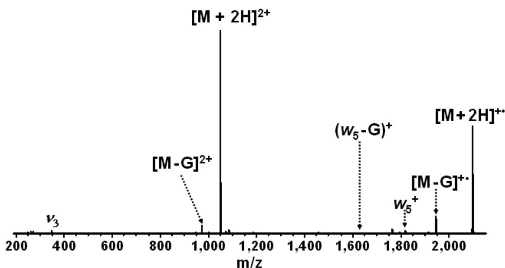
Figure 6-3. ECD (-1 V bias voltage, 40 ms, 50 scans) of doubly protonated 2'-methoxy  $G_6$ . Product ions labeled  $w$  can also be  $d$  ions. Abundant charge reduced precursor ions are detected.
