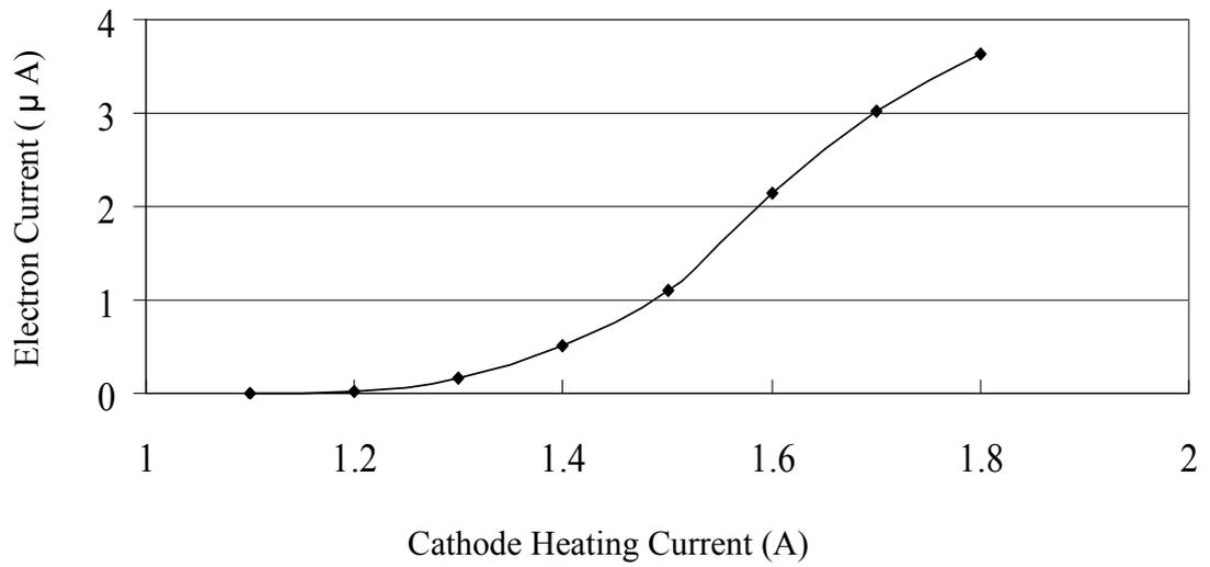
Figure 3-6. Electron current passing through the ICR cell as a function of cathode heating current at fixed cathode bias voltage (- 18.0 V) and extraction lens voltage (- 19.0 V).
