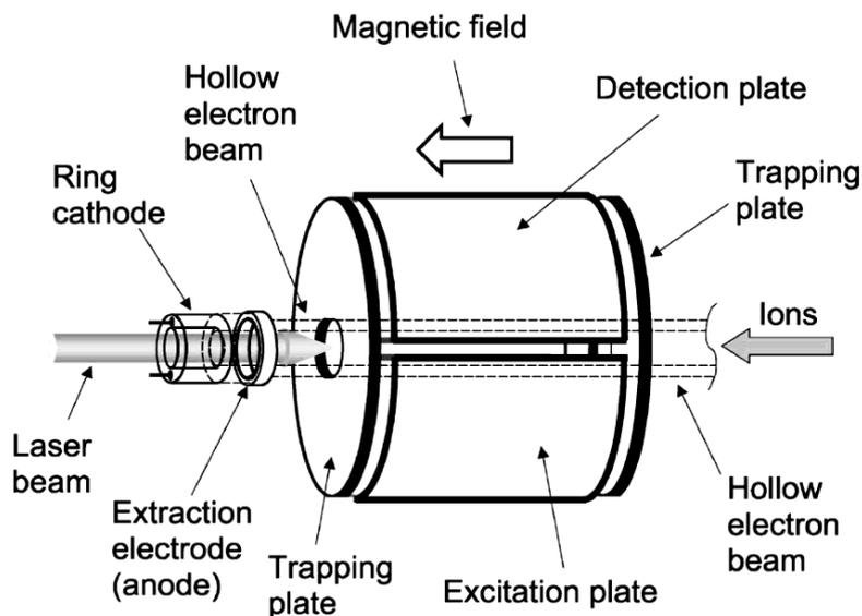
Figure 2-3. Schematic diagram of an indirectly heated hollow dispenser cathode EDD configuration. This figure is reproduced from reference [12] with permission.
