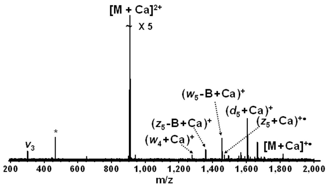
Figure A-5. ECD (1 eV electrons, 30 ms, 50 scans) of  $[d(GCATAC) + Ca]^{2+}$ . Electronic noise spike is labeled with an asterisk,  $v_3$  = harmonic artifact.
