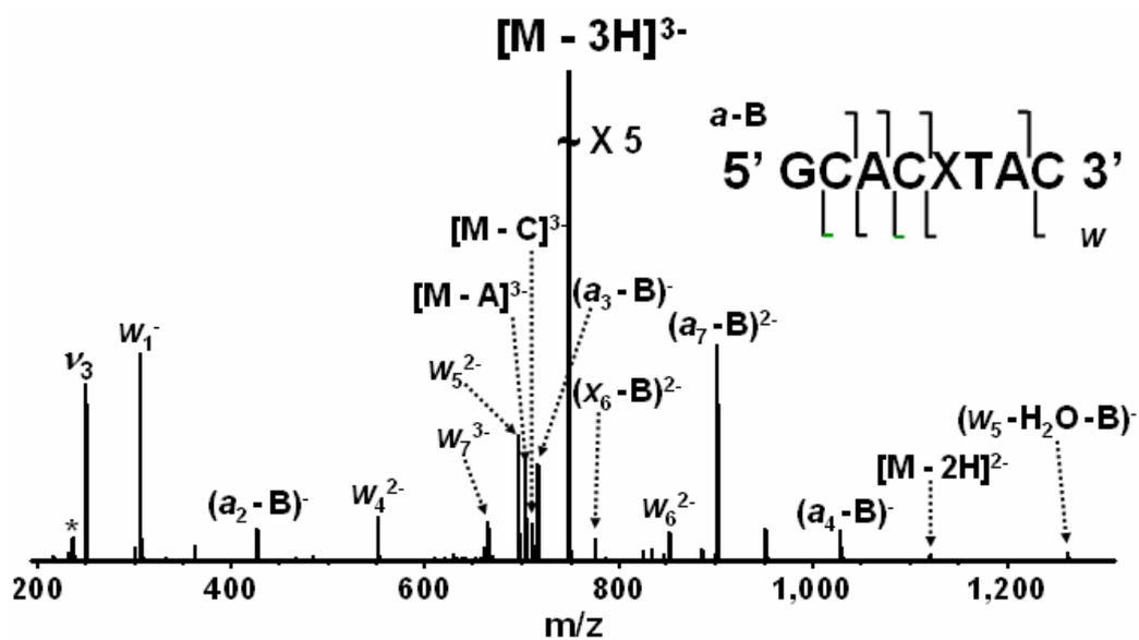
Figure 6-20. IRMPD (10.6  $\mu$ m, 25 ms irradiation at 7.5 W laser power, 50 scans) of triply deprotonated d(GCACXTAC) (X denotes an abasic site at which a nucleobase has been replaced by hydrogen). Observed backbone bond cleavages are summarized in the inset.
