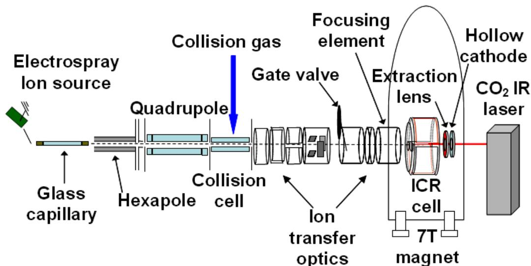
Figure 2-1. Schematic diagram of our 7 T ESI-Q-FT-ICR mass spectrometer.
