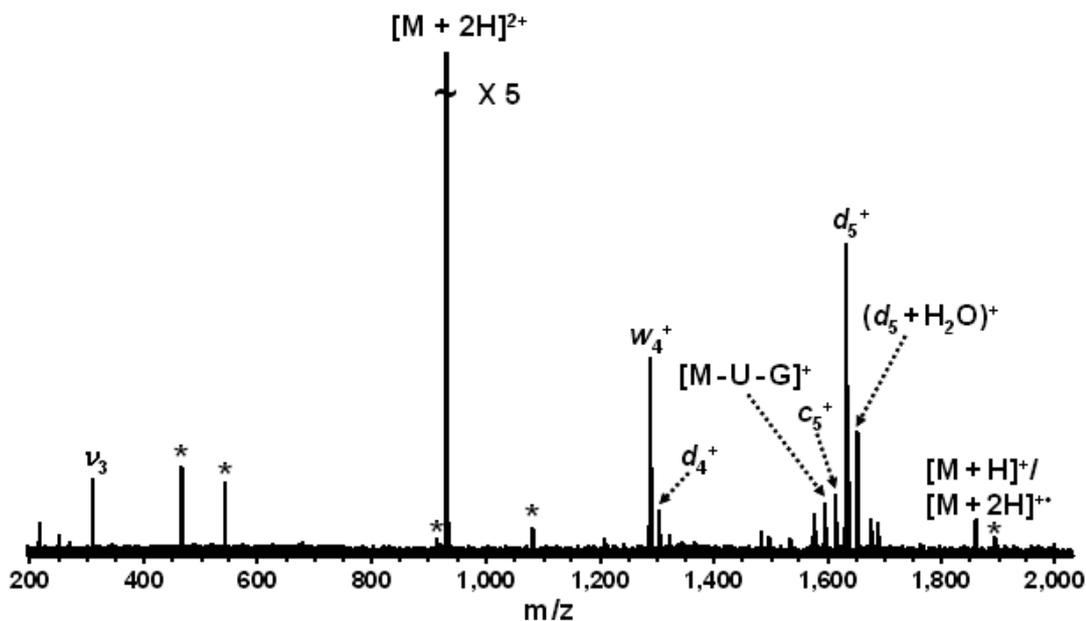
Figure 4-4. ECD (- 1 V bias voltage, 35 ms irradiation, 32 scans) of the RNA GCAUAC.
