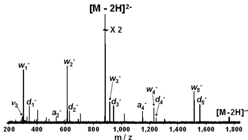
Figure 6-17. EDD (-18.2 V, 2 s, 30 scans) of doubly deprotonated methylphosphonate-containing d(GCATAC). Complete  $d$  and  $w$  ion series, together with two complementary  $a$  ions are observed, allowing full sequencing of the oligonucleotide.
