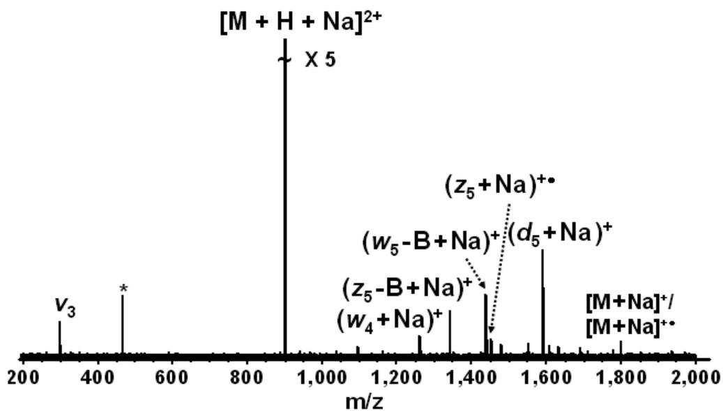
Figure A-2. ECD (1 eV electrons, 25 ms, 50 scans) of  $[d(GCATAC) + H + Na]^{2+}$ .
