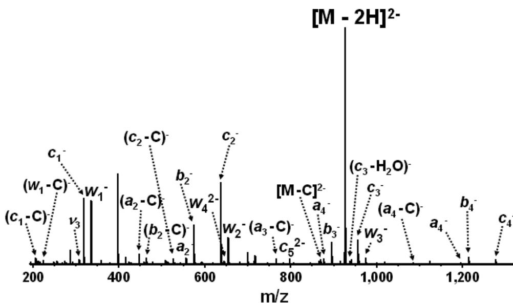
Figure 6-6. IRMPD (10.6  $\mu\text{m}$ , 45 ms irradiation at 7.5 W laser power, 50 scans) of doubly deprotonated 2'-methoxy  $\text{C}_6$ . Ions labeled  $b$  can also be  $y$  ions, and ions labeled  $c$  can also be  $x$  ions. A complete  $c/x$  ion series allowed full sequencing of the oligonucleotide.
