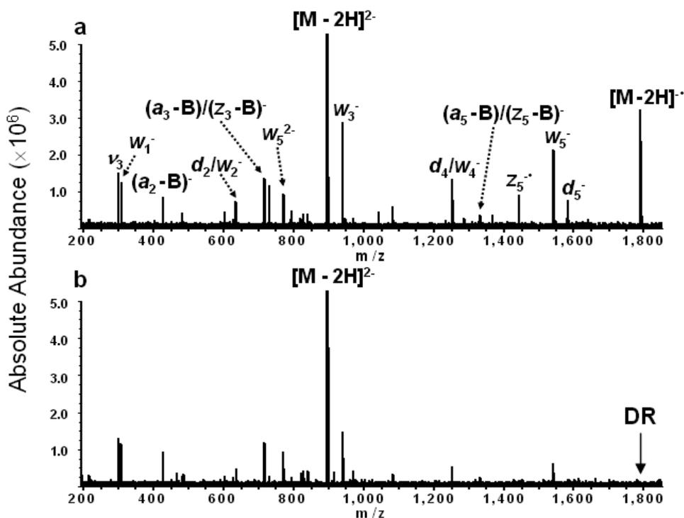
Figure 5-9. EDD spectra of doubly deprotonated d(GCATGC) without DR (a) and with DR ejection at the frequency of  $[M - 2H]^-$  (b). (the solid arrow indicates the  $m/z$  value corresponding to the frequency of the DR rf waveform).
