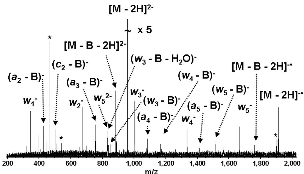
Figure 2-7. EDD (17 eV electrons, 1 s irradiation, 30 scans) of  $dG_6$  with an indirectly heated hollow dispenser cathode electron source. The spectrum is similar to EDD of  $dA_6$  and  $dC_6$ , see Figures 2-5 and 2-6. However, no  $a/z$ , or  $c/x$  ions are observed, correlating with the labile nature of guanine. Only one label is given for  $d/w$ ,  $c/x$  and  $a/z$  ion series. Electronic noise spikes are labeled with asterisks.
