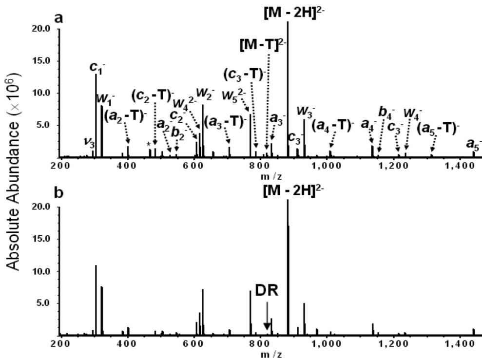
Figure 5-3. IRMPD spectra of doubly deprotonated  $dT_6$  without (a) and with (b) DR ejection at the ICR frequency of  $[M - T]^{2-}$ . (The solid arrow indicates the  $m/z$  corresponding to the frequency of the DR rf waveform, \* = electronic noise spike).
