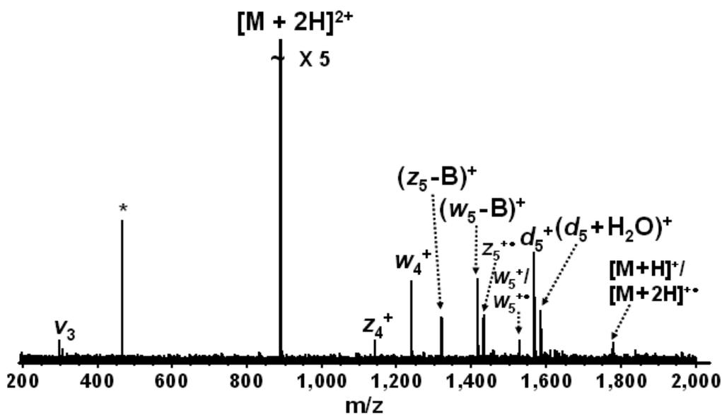
Figure A-1. ECD (1 eV electrons, 30 ms, 50 scans) of doubly protonated d(GCATAC).
