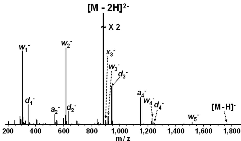
Figure 6-18. IRMPD (10.6  $\mu\text{m}$ , 18 ms irradiation at 7.5 W laser power, 30 scans) of doubly deprotonated methylphosphonate-containing d(GCATAC). A complete  $w$  ion series provides full sequence coverage.
