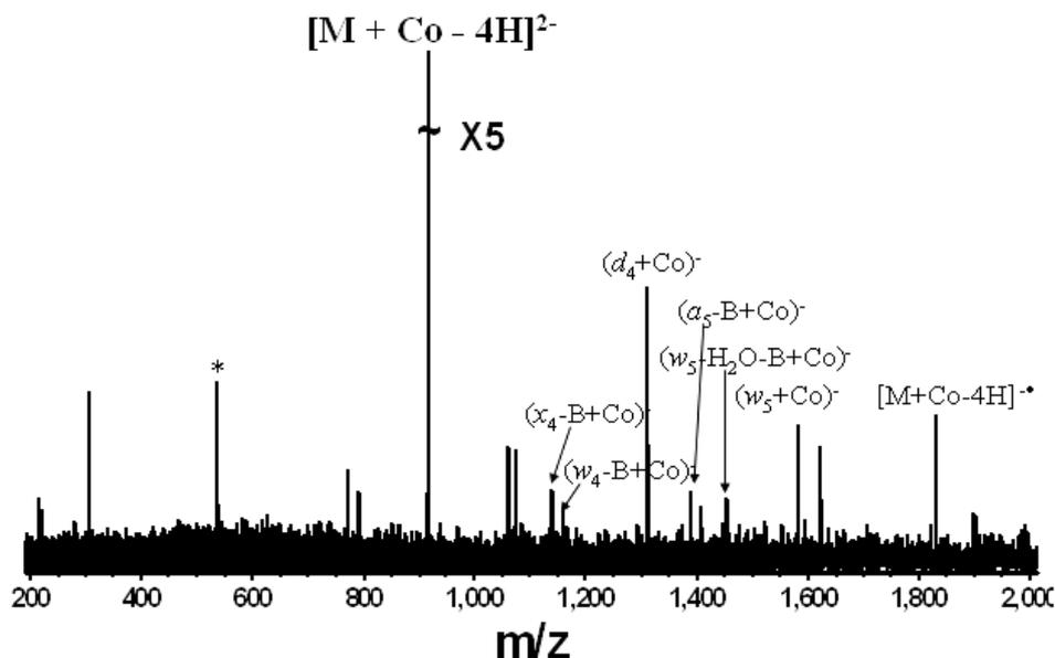
Figure A-13. EDD (18.2 eV electrons, 2 s, 15 scans) of  $[d(\text{GCATAC}) + \text{Co} - 4\text{H}]^{2-}$ .
