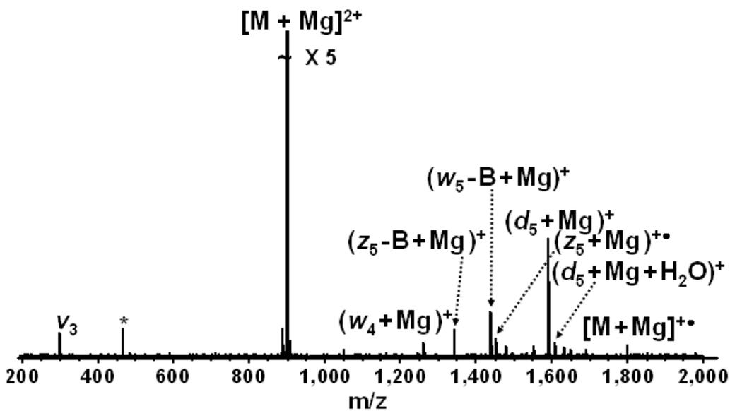
Figure A-4. ECD (1 eV electrons, 25 ms, 50 scans) of  $[d(\text{GCATAC}) + \text{Mg}]^{2+}$ . Electronic
