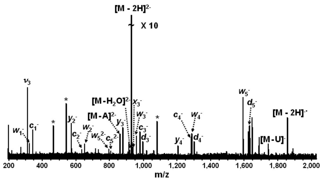
Figure 4-10. EDD (- 18.2 V bias voltage, 2 s irradiation, 32 scans) of the RNA GCAUAC. A complete  $w$  ion series is observed, allowing full sequencing of the oligonucleotide. Electronic noise spikes are labeled with asterisks.
