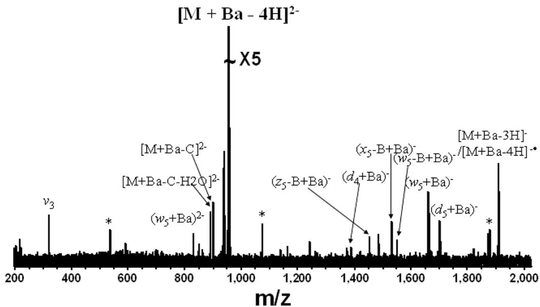
Figure A-12. EDD (18.2 eV electrons, 2 s, 32 scans) of  $[d(\text{GCATAC}) + \text{Ba} - 4\text{H}]^{2-}$ .
