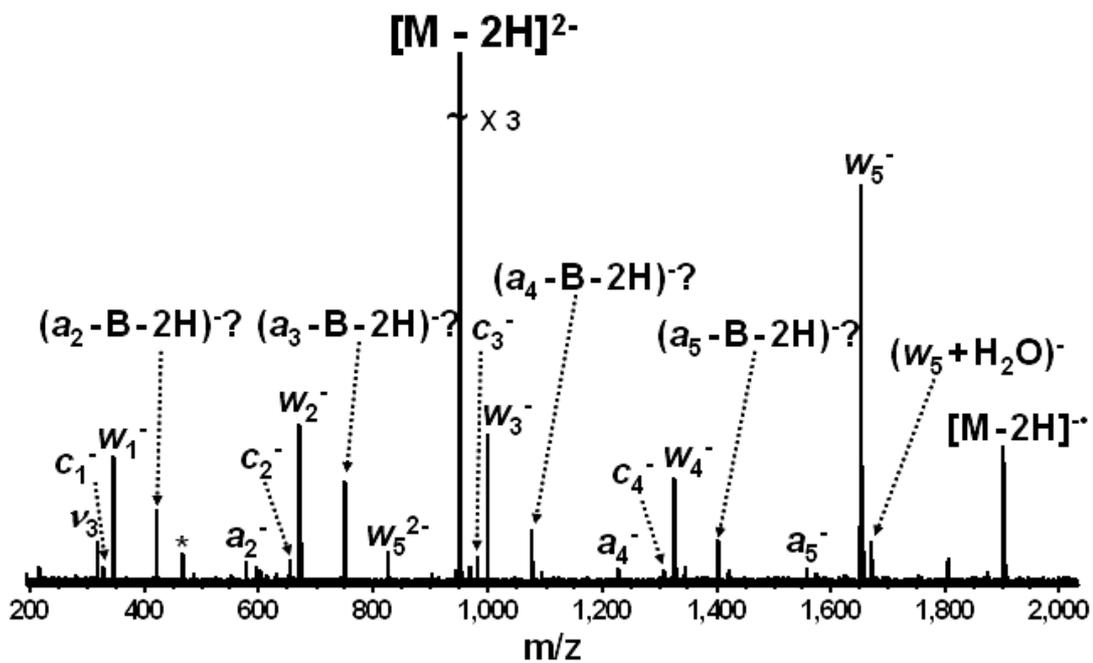
Figure 6-15. EDD of doubly deprotonated methylphosphonate-containing  $dG_6$ . Product ions labeled  $w$  can also be  $d$  ions, ions labeled  $a$  can also be  $z$  ions, and ions labeled  $c$  can also be  $x$  ions. A complete series of  $d/w$  ions is observed, allowing full sequencing of the oligonucleotide. Question marks denote assignments with high (>20 ppm) mass error. Electronic noise spike is labeled with an asterisk.
