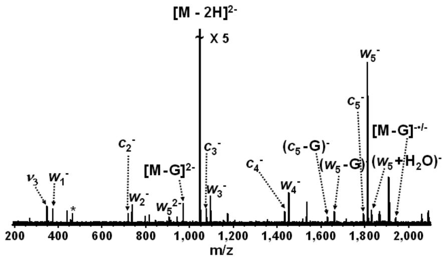
Figure 6-8. EDD (-18.2 V, 2 s, 50 scans) of doubly deprotonated 2'-methoxy G<sub>6</sub>. Product ions labeled *w* can also be *d* ions, and ions labeled *c* can also be *x* ions. Full series of *d/w* ions are observed, allowing full sequencing of the oligonucleotide. Electronic noise spike is labeled with an asterisk.
