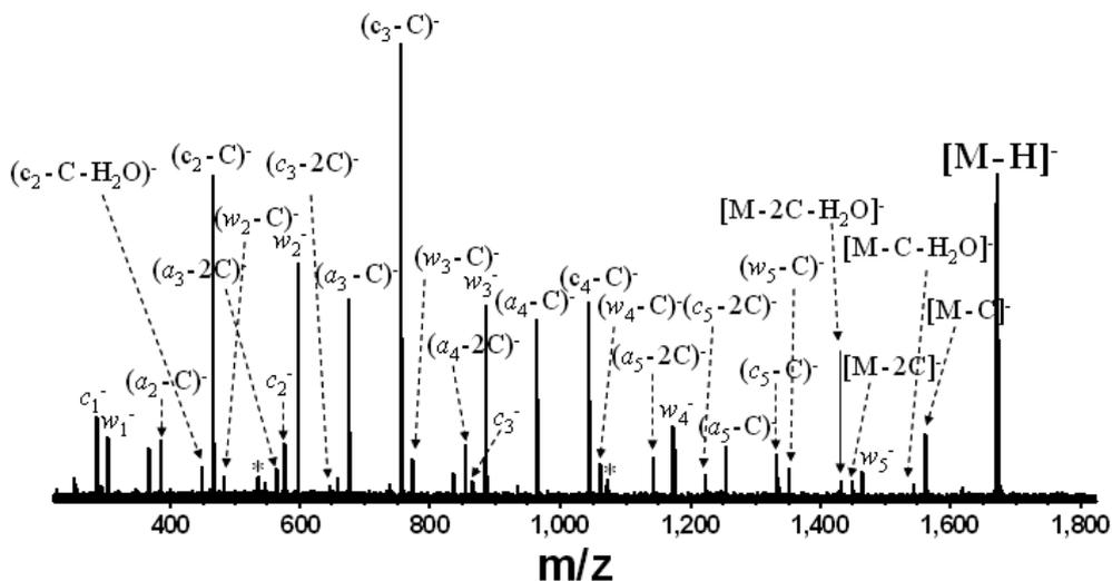
Figure B-4. IRMPD (10 W, 20 ms, 32 scans) of singly deprotonated  $dC_6$ . Mainly  $c/x$ ,  $d/w$ ,  $(a/z - B)$ ,  $(d/w - B)$ , and  $(c/x - B)$  ions are observed. Electronic noise spikes are labeled with asterisks.
