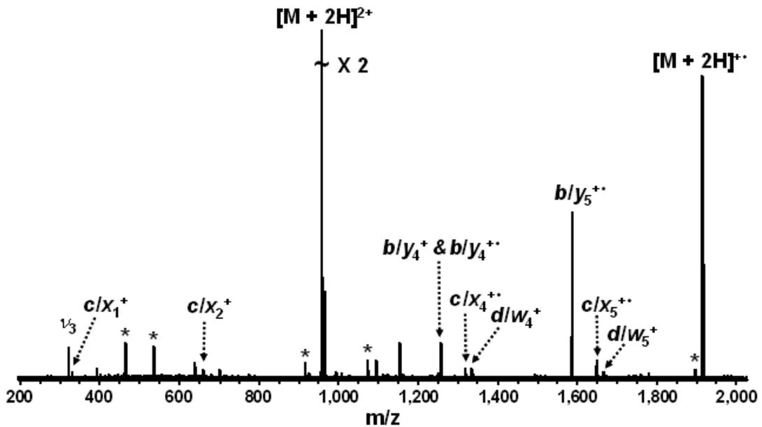
Figure 4-1. ECD (- 1 V bias voltage, 80 ms irradiation, 32 scans) of the RNA  $A_6$ .  $b/y$ ,  $c/x$  and  $d/w$  ions are observed in addition to an abundant charged reduced radical species,  $[M + 2H]^{+•}$ . Electronic noise spikes are labeled with asterisks.
