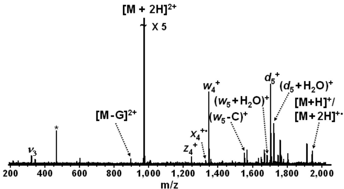
Figure 6-4. ECD (-1 V bias voltage, 35 ms, 50 scans) of doubly protonated 2'-methoxy GCAUAC. Electronic noise spike is labeled with an asterisk.
