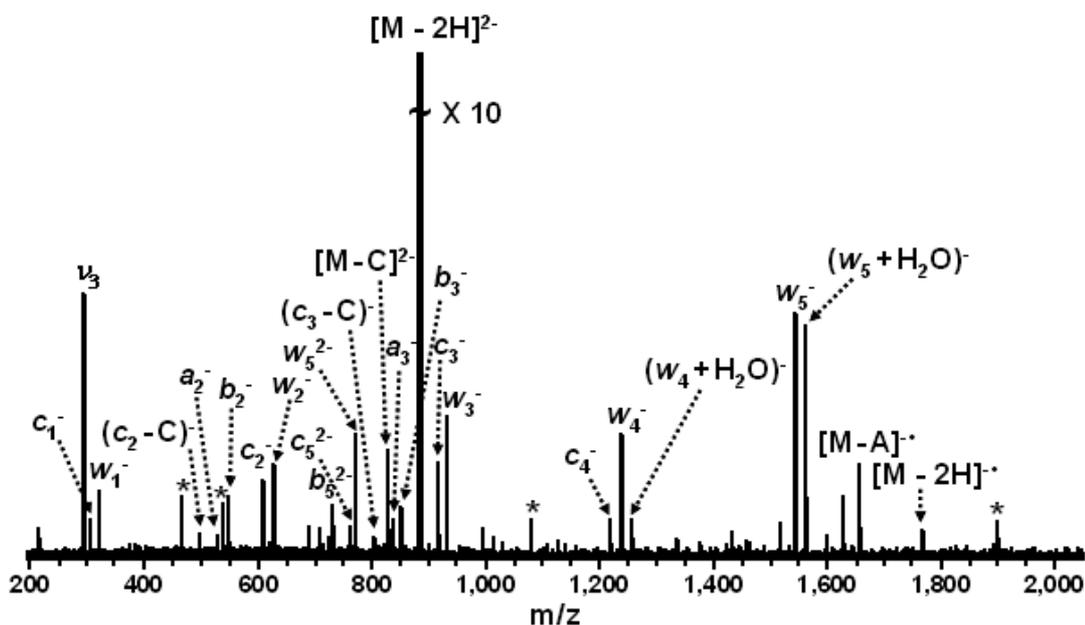
Figure 4-6. EDD (- 18.1 V bias voltage, 2 s irradiation, 32 scans) of the RNA C<sub>6</sub>. A complete *d/w* ion series is observed, allowing full sequencing of the oligonucleotide. Electronic noise spikes are labeled with asterisks.
