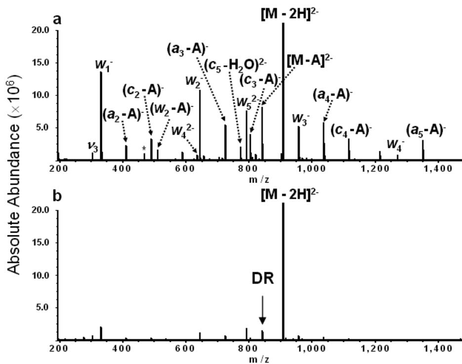
Figure 5-1. IRMPD spectra of doubly deprotonated  $dA_6$  without (a) and with (b) double resonance ejection at the ICR frequency of  $[M - A]^{2-}$ . (The solid arrow indicates the  $m/z$  corresponding to the frequency of the DR rf waveform, \* = electronic noise spike).
