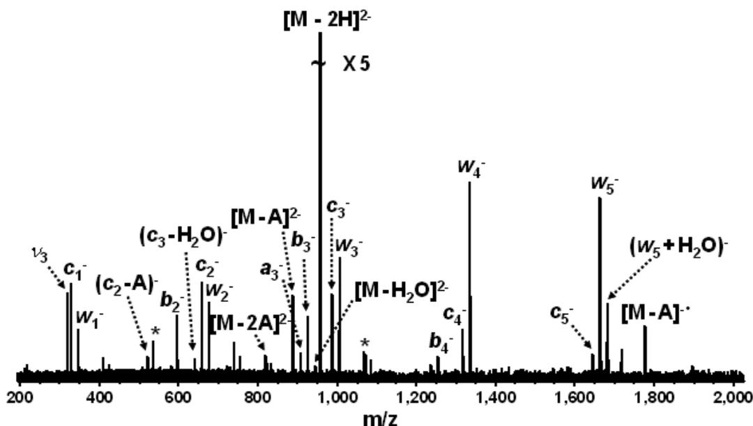
Figure 4-5. EDD (- 18.1 V bias voltage, 2 s irradiation, 32 scans) of the RNA A<sub>6</sub>. Complete *d/w* and *c/x* ion series are observed (only one of the labels is given), allowing full sequencing of the oligonucleotide. Electronic noise spikes are labeled with asterisks.
