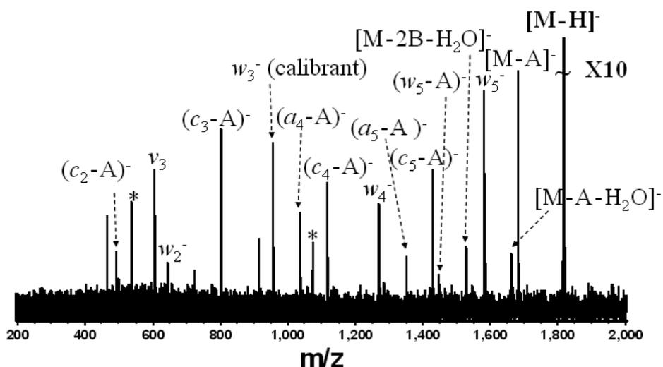
Figure B-1. EID (18.1 eV electrons, 2 s, 32 scans) of singly deprotonated  $dA_6$ .  $d/w$ ,  $(a/z - B)$ ,  $(d/w - B)$  and  $(c/x - B)$  ions are observed (only one of the labels is given). Electronic noise spikes are labeled with asterisks.
