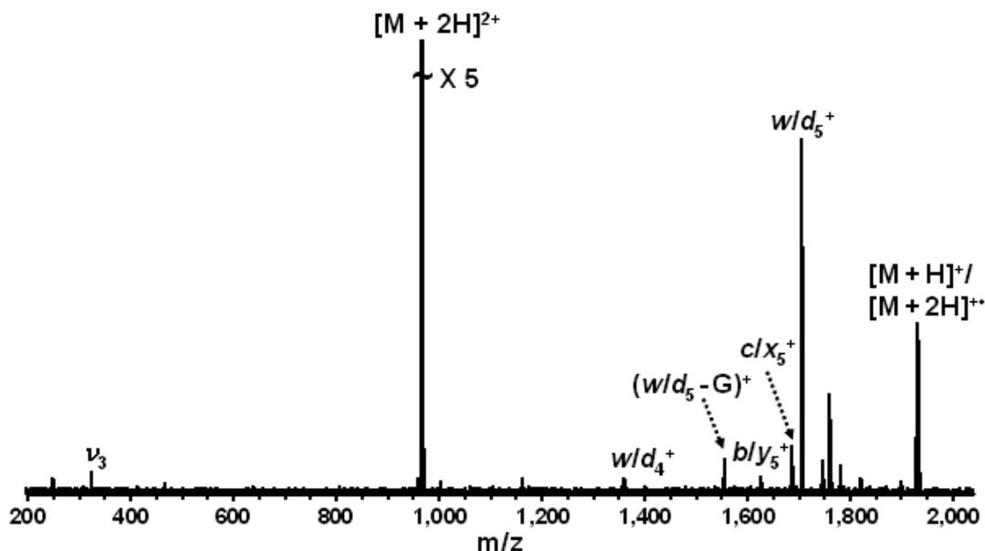
Figure 4-3. ECD (- 1 V bias voltage, 70 ms irradiation, 50 scans) of the RNA CGGGGC. Incomplete  $w/d$ ,  $c/x$ ,  $b/y$ , and  $(w/d - G)$  ion series are present.
