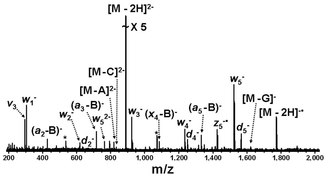
Figure 2-10. EDD of d(GCATAC) (2 s irradiation, - 18.1 V bias, 32 scans) results in a complete  $w$  ion series, and three  $d$  ions. The latter ions are generally not observed in tandem mass spectrometry, such as CAD and IRMPD. Electronic noise spikes are labeled with asterisks.
