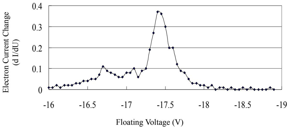
Figure 3-7. Electron energy distribution at -19.0 V cathode bias voltage, -19.0 V extraction lens voltage, and 1.2 A heating current.
