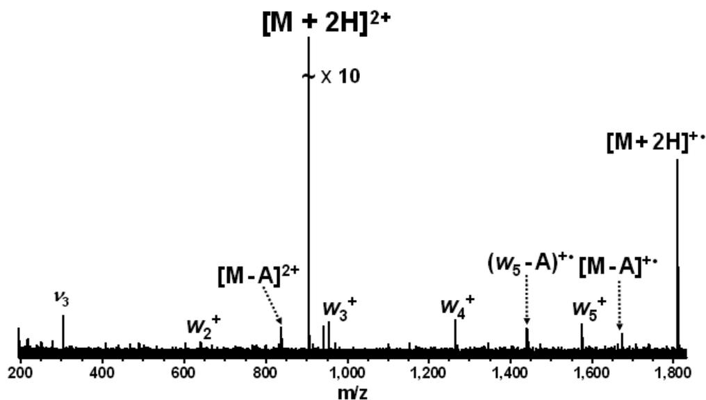
Figure 6-10. ECD (- 1 V bias voltage, 20 ms, 32 scans) of doubly protonated methylphosphonate-containing  $dA_6$ .  $d/w$  ions are labeled as  $w$  ions.
