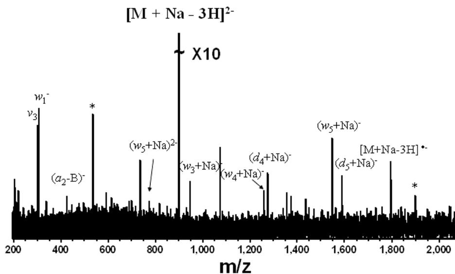
Figure A-8. EDD (18.2 eV electrons, 2 s, 32 scans) of  $[d(GCATAC) + Na - 3H]^{2-}$ . Electronic noise spikes are labeled with asterisks,  $v_3$  = harmonic artifact.
