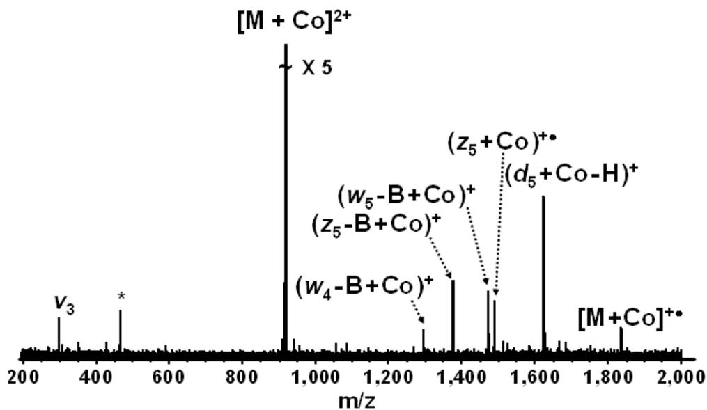
Figure A-6. ECD (1 eV electrons, 25 ms, 50 scans) of  $[d(GCATAC) + Co]^{2+}$ . Electronic noise spike is labeled with an asterisk,  $v_3$  = harmonic artifact.
