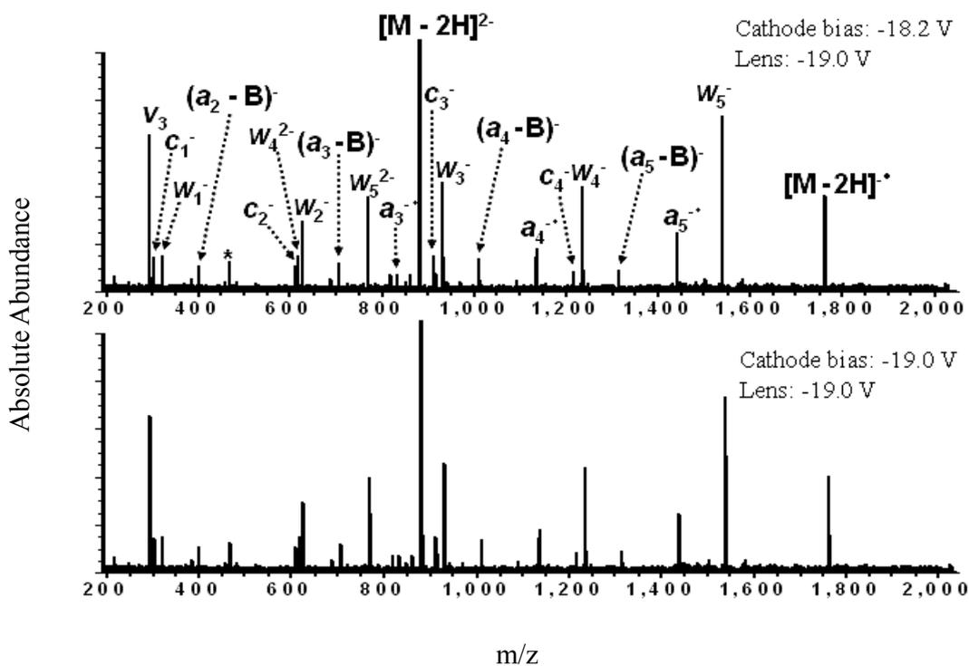
Figure 3-8. EDD spectra (same scale) of the oligonucleotide  $dT_6$  at different cathode heating current: 1.8 A (top) and 1.2 A (bottom) but at fixed electron current passing through the ICR cell. (\* = electronic noise).
