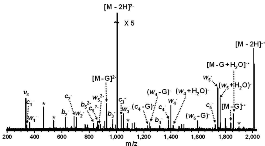
Figure 4-7. EDD (- 18.3 V bias voltage, 2 s irradiation, 32 scans) of the RNA  $G_6$ . Complete  $d/w$  and  $c/x$  ion series are observed, allowing full sequencing of the oligonucleotide. Electronic noise spikes are labeled with asterisks.
