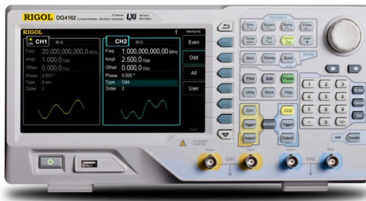
Figure 7: Rigol DG 4102 Function Generator used to deliver an electric field with varying frequencies and voltages across the liquid-liquid interface
