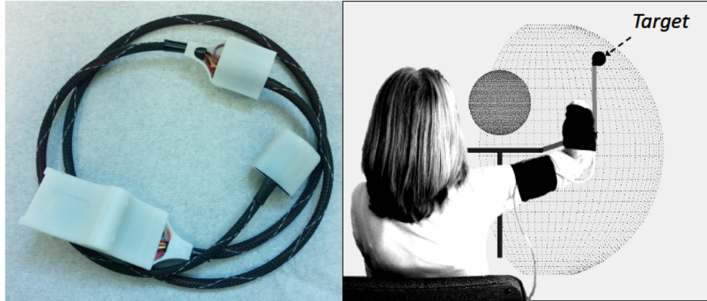
Figure A.2: The completed IMU system (left). Use of the IMU system being worn by an amputee subject (right). The amputee subject is viewing an image of her limb's orientation as estimated by the IMU system.
