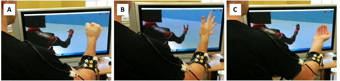
Figure 1.3: Images showing the testing of a pattern recognition system in a virtual environment where (A) shows a hand close grasp, (B) shows a hand open grasp, and (C) shows a wrist supinate grasp. The hand is controlled in the virtual environment by means of EMG pattern recognition. The arm is controlled in the virtual environment by means of the inertial measurement units (IMUs) worn by the subject as described in Appendix A.
