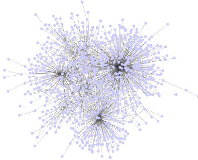
Figure 9: An example of a scale-free network. Notice there are a few highly connected node called hubs and many nodes of low degree connected to the hubs.
