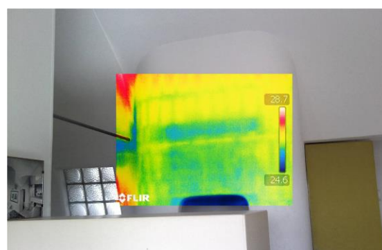
Figure 5. © A-BIME: Infrared camera picture: structure of the shower wall
