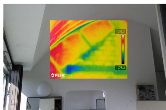
Figure 4. © A-BIME: Infrared camera picture: structure of the bedroom wall
