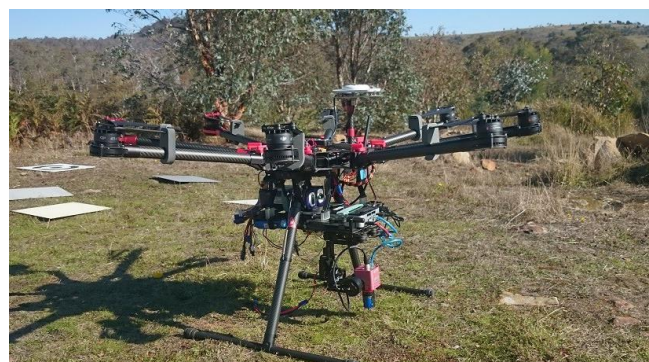
Figure 1. The DJI S-1000 multi-rotor flight platform, with downward facing PhotonFocus camera attached to the 2-axis gimbal and Trimble GNSS receiver mounted on top.
