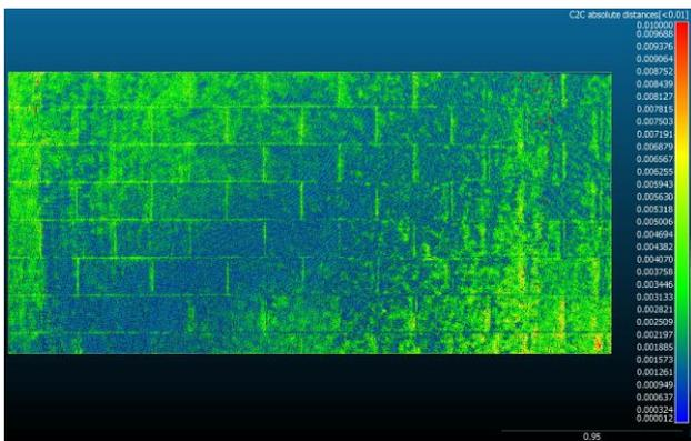
Figure 6. Comparison between a laser scan and the photogrammetric point cloud generated from central perspective images in the room with check points.
