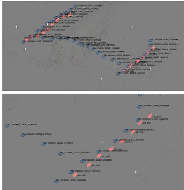
Figure 5. Image orientation results for central perspectives and 360° images in the two rooms (top), and a detail for only the second room (bottom).
