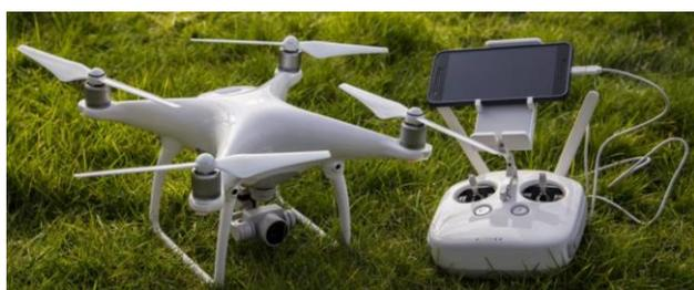
Figure 21. UAV-Photogrammetric Drone System – Phantom 4 DJI System
