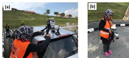
Figure 7. Mobile laser scanning (a) vehicle-based mode and (b) human-based mode
