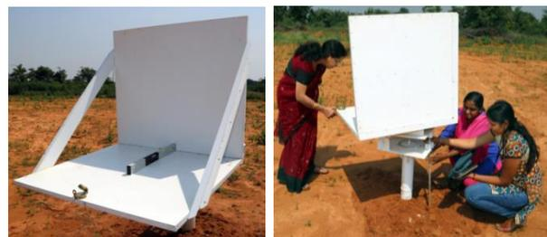
Figure 1: Corner Reflectors deployed at NRSC Microwave Cal-Val site
