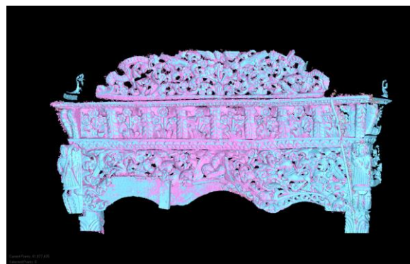
Fig. 6a Point-to-point comparison between the SfM and laser clouds
