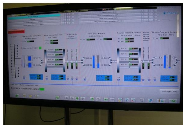
Figure 6. SCADA system main water pipelines
