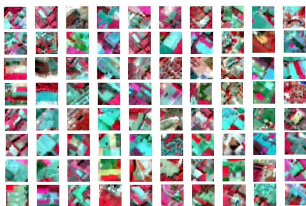
Figure 4. Built-up area patches generated from Sentinel-2 dataset for training and testing networks
