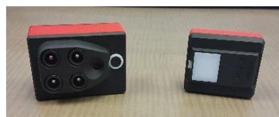
(a): The Sequoia camera on the left, while the GPS /IMU sensor on the right.
