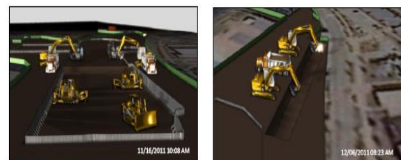
(a) Screenshots of 4D excavation simulations depicting installation of sheet piles and utility pipes.
