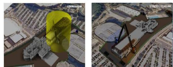
(b) Crane work zone and steel truss placement in the crane management plan.
