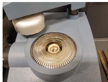
Fig. 8 Specimen loaded in DSC's chamber
