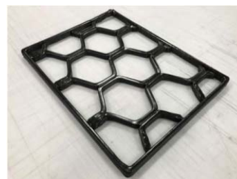
Fig. 1 Prototype 3D printed recycled carbon fiber part
