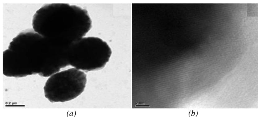
Fig. 1. TEM images of (a) spherical  $\text{Fe}_3\text{O}_4$  and (b) HRM image of atomic layers.
