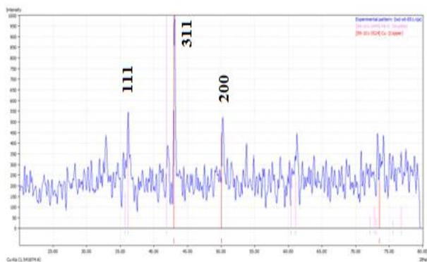
Fig. 2. XRD plots of Sol-Gel prepared  $Fe_3O_4$  particles.
