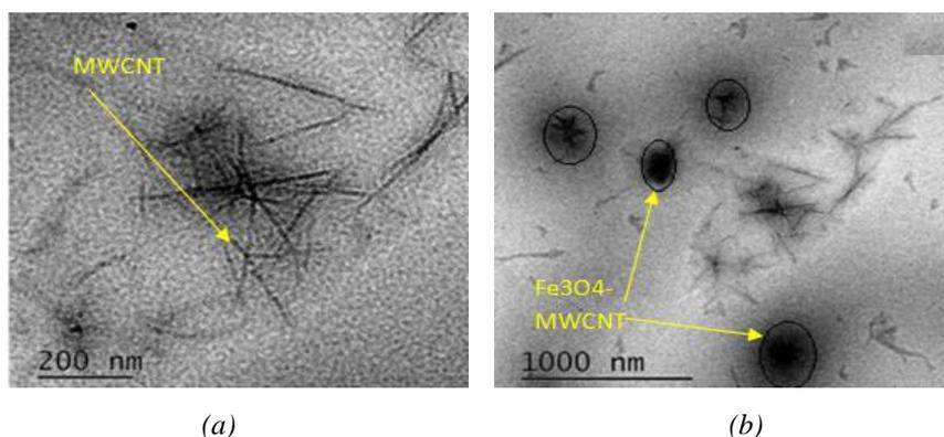
Fig. 3. TEM images of (a) MWCNT and (b) MWCNT- $Fe_3O_4$  compound.
