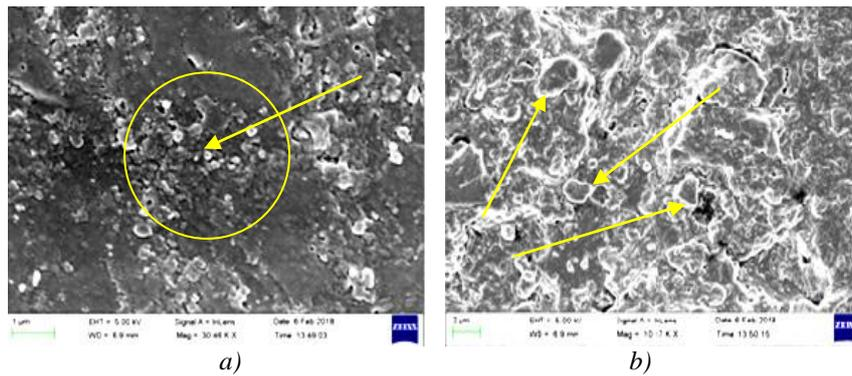
Fig. 8. (a & b) SEM images of MWCNT with  $Fe_3O_4$  in rubber matrix.
