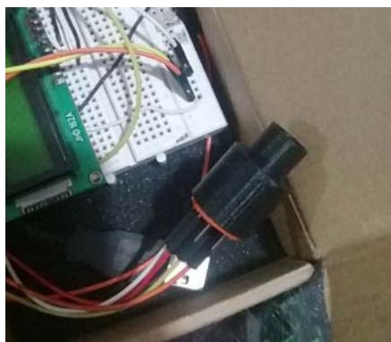
Fig. 3 Mouthpiece with MQ 138 sensor
