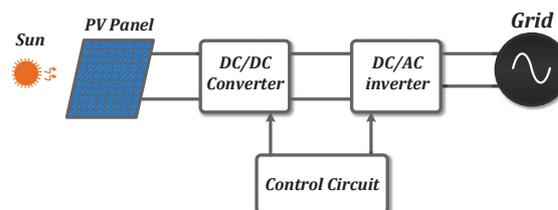
Fig. 1 Block Diagram of Grid-Connected PV Systems
