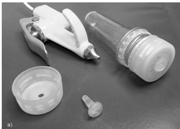
Figure 5. a) Pressurizable polypropylene bottles, cups, valves and dispenser used in the experiments, b) atelocollagen dry powder dissolution kinetics – AA 0.1 M (triangles), AA 0.5 M (circles), CO 2 0.5 MPa (stars), CO 2 0.9 MPa (diamonds).
