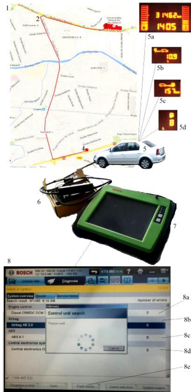
Fig. 2. Experimental set for ECU-KTS communication 1-experiment site map; 2-track, 3-start-point; 4-end-point; 5- tested vehicle; 5a-ON-BOARD display with total number of km; 5b-consumed fuel quantity during tests; 5c-mileage; 5d-fuel quantity in the vehicle's tank; 6-analog-digital converter; 7-KTS-Bosch 650; 8-graphic interface; 8a-engine module link; 8b-airbag; 8c-Anti-lock Braking System; 8d-fault details.
