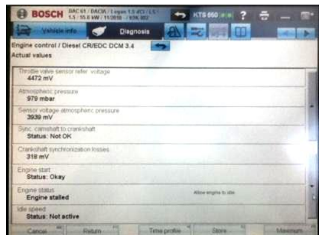
Fig. 8. Actual values for throttle valve and crankshaft sensors
