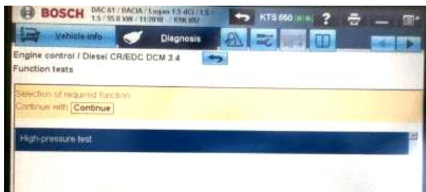
Fig. 16. Access of the high pressure test in CR system
