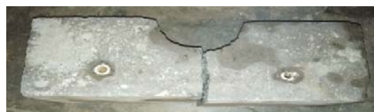
Fig. 7 Concrete block after flexural strength
