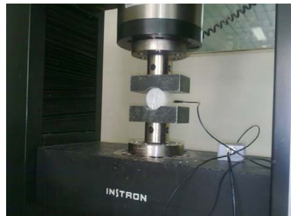
Fig. 2 Servo-electric loading frame with AE monitoring system
