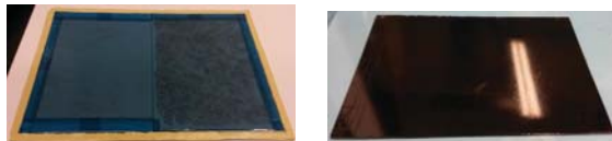
(a) Film Seal and Tape Dam (b) Contained Cure Outcome
