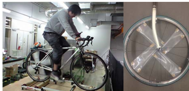
Fig. 1 Bicycle with Wells turbine in wheels
