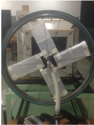
Fig. 3 Wells turbine in a wheel
