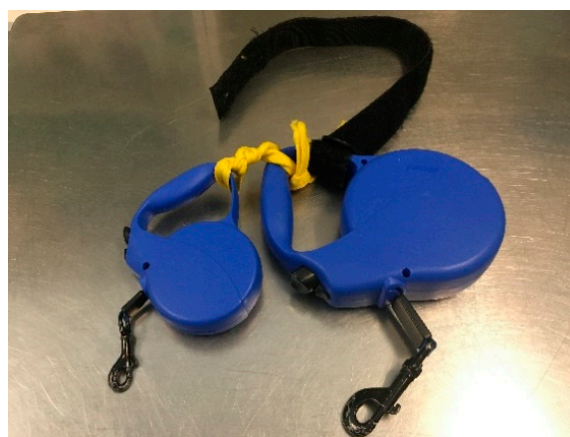
Figure 1. Two retractable Flexi (TM) compact leads attached together with velcro tie in preparation for mounting.
