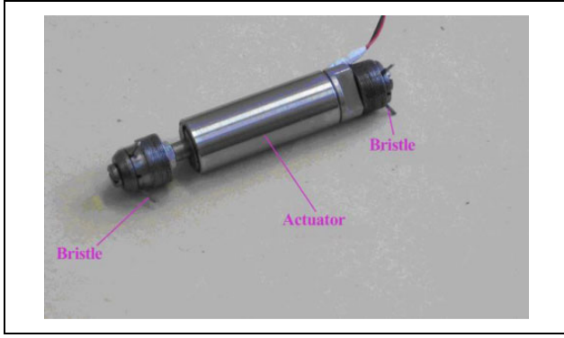
Figure 1. Bristled in-pipe robot.
