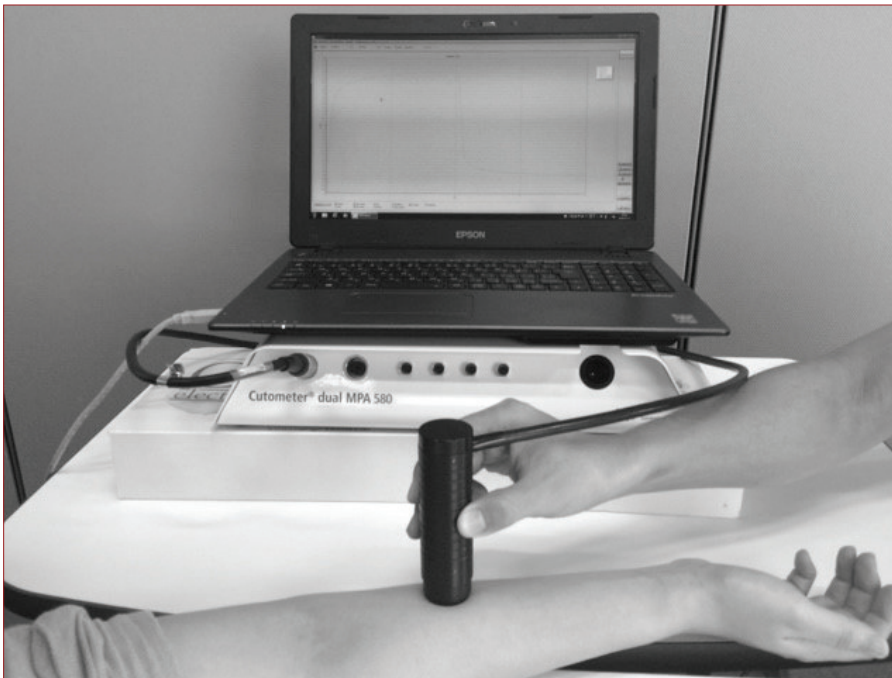
FIGURE 1. Skin viscoelasticity measurements were obtained by using a Cutometer MPA 580®.
