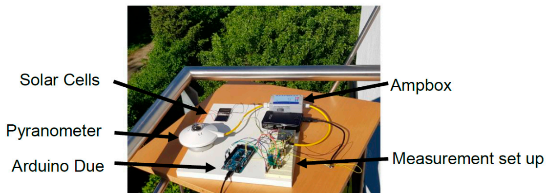
Figure 4. Picture of the setup placed onto a sunny balcony.
