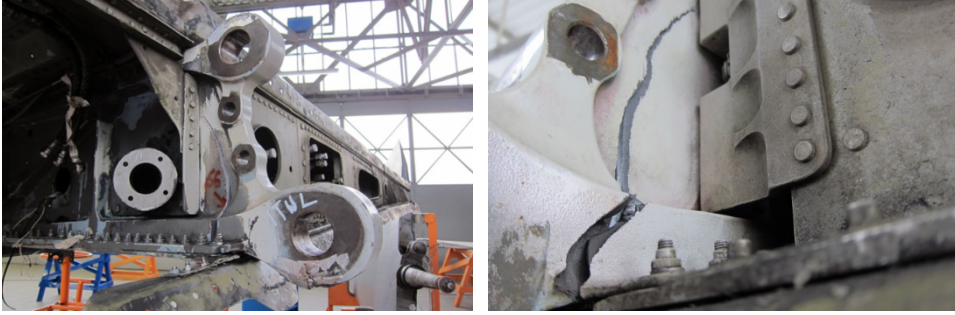
Fig. 1. Critical damage in the Full Scale Durability Test
