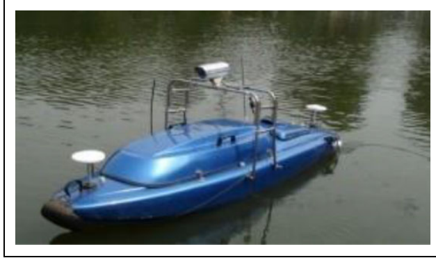
Figure 6. The USV system in our experiments. USV: unmanned surface vehicle.
