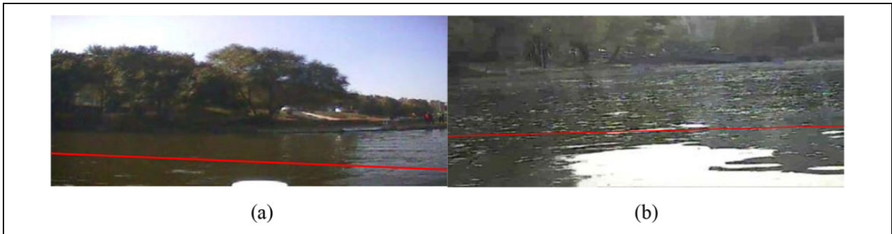
Figure 16. Waterline detection result with the traditional gray image and the shadow detection method using the image in Figures 7(a) and 11(a). (a) Waterline detection with the traditional gray image for Figure 7(a) and (b) Waterline detection with shadow detection for Figure 11(a).
