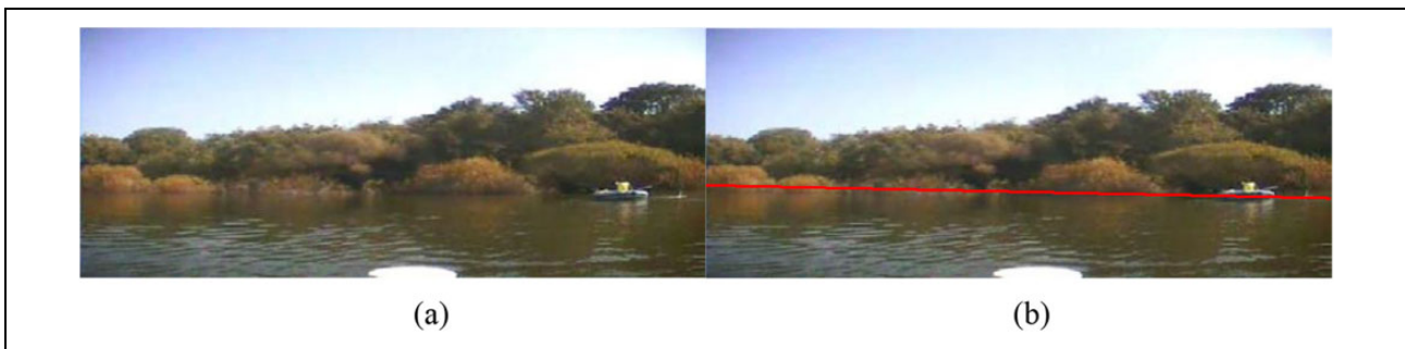
Figure 9. Waterline detection result for cast shadow colors close to colors of the cast objects on the bank. (a) The original image before waterline detection and (b) The image after waterline detection.
