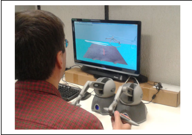
Figure 22. User performing a simple suturing task in SutureHap.
