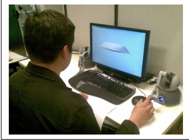
Figure 20. User performing the haptic perception test of the skin on the simulation, implemented on a NVIDIA PhysX cloth model.
