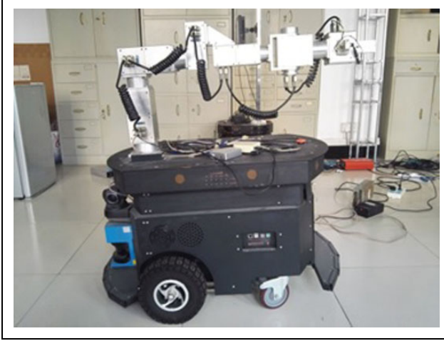
Figure 1. Six-DOF Stanford MT-ARM robotic manipulator. DOF: degree of freedom.
