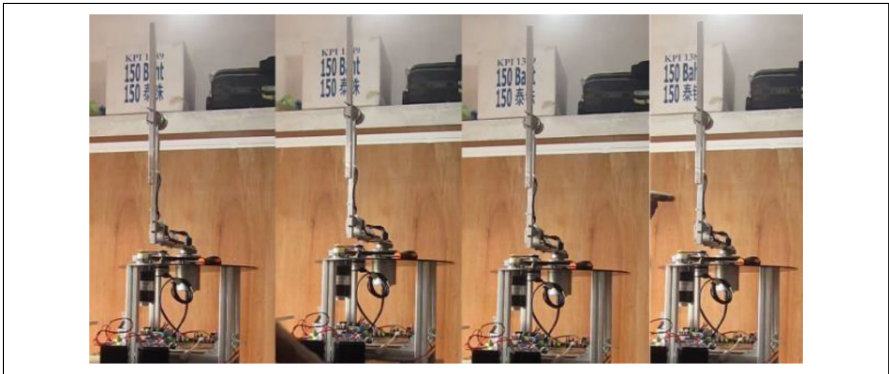
Figure 27. Snapshots from balancing experiment of RDIP system. RDIP: rotary double inverted pendulum.
