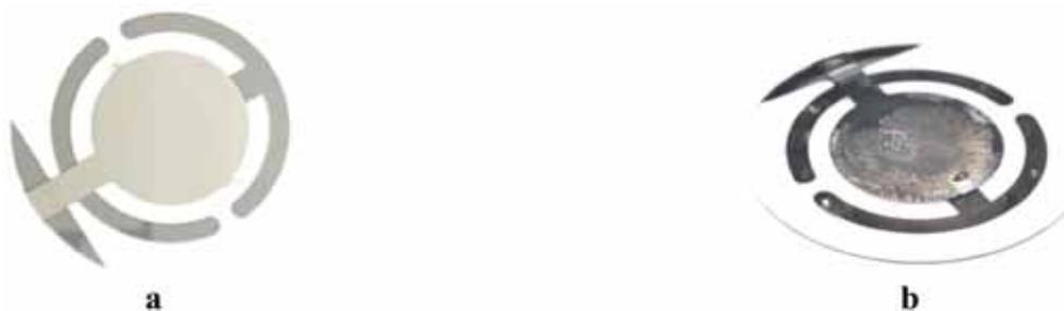
**Figure 1.** QCM sensor (a) before and (b) after adsorption process.
