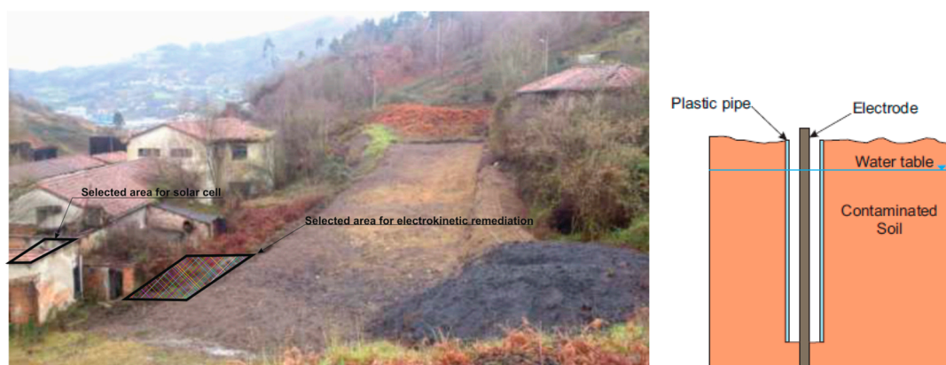
Figure 2. View of selected area for electrokinetic remediation field study and scheme of electrode.
