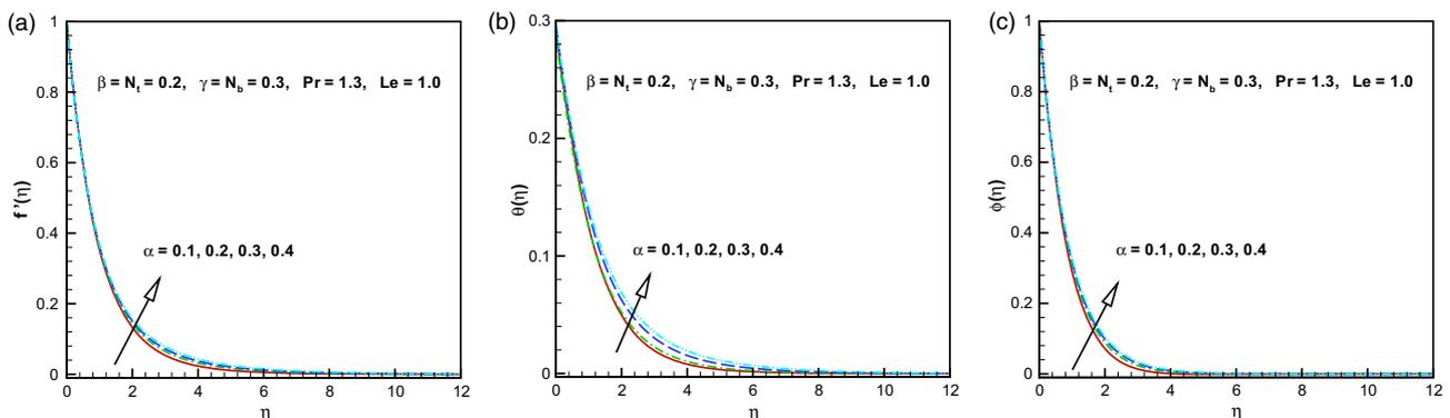
**Figure 2.** Influence of the curvature parameter  $\alpha$  on (a) velocity, (b) temperature and (c) concentration fields.
