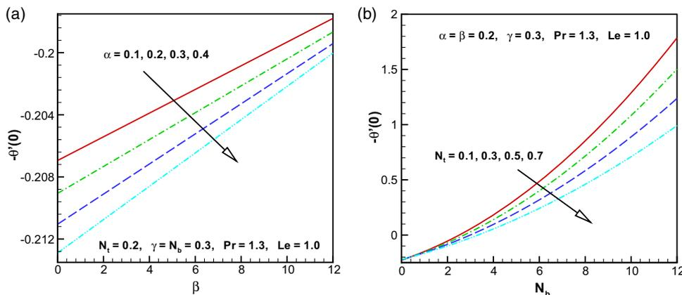
Figure 8. Influence of the curvature parameter  $\alpha$  (a) and thermophoresis parameter  $N_t$  (b) on Nusselt number.
