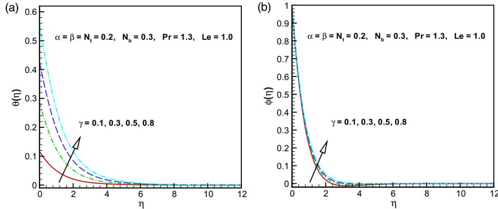
Figure 6. Influence of the Biot number  $\gamma$  on (a) temperature and (b) concentration fields.
