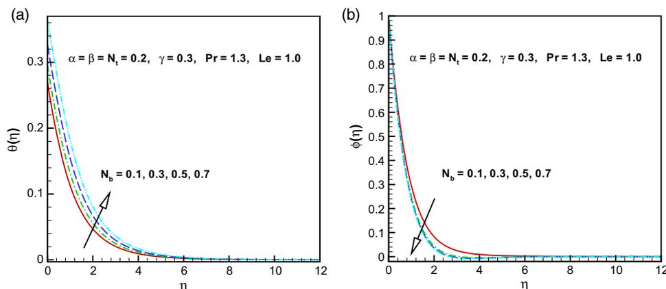
**Figure 5.** Influence of the Brownian motion parameter  $N_b$  on (a) temperature and (b) concentration fields.
