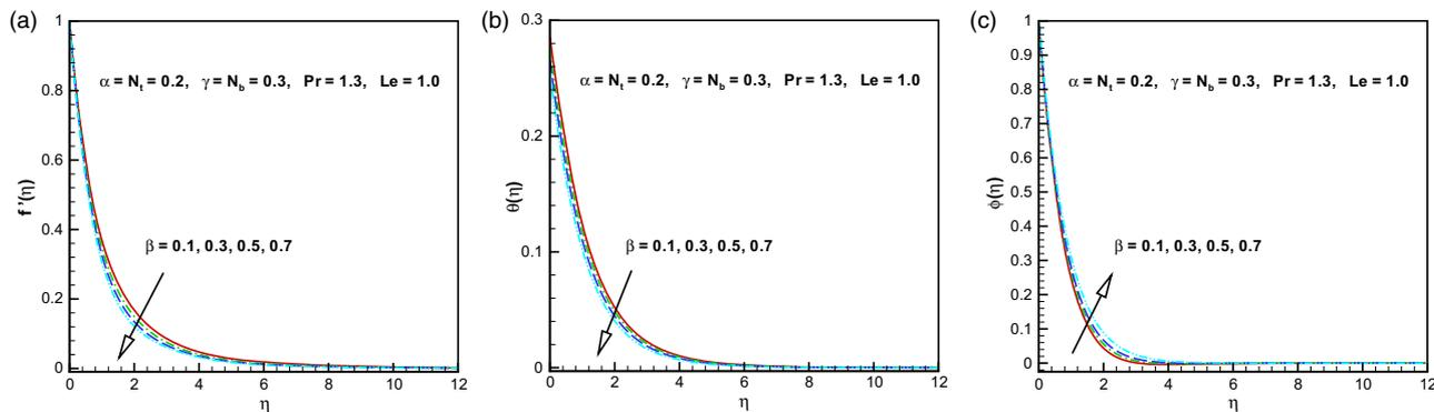
**Figure 3.** Influence of the Deborah number  $\beta$  on (a) velocity, (b) temperature and (c) concentration fields.
