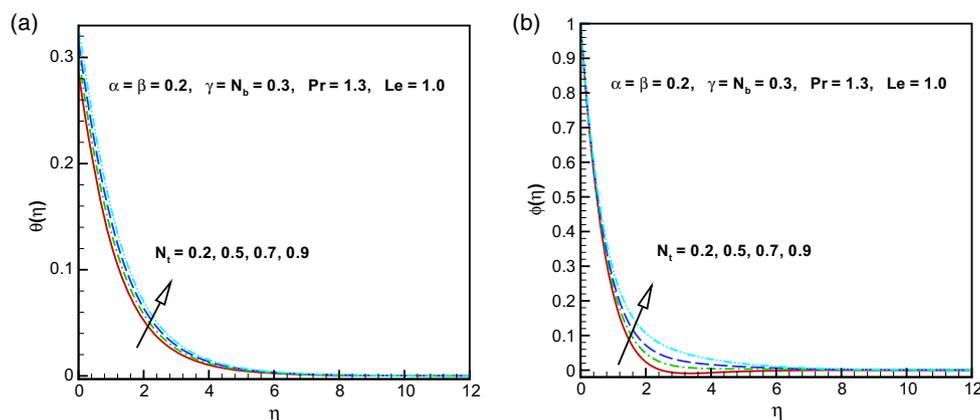
**Figure 4.** Influence of the thermophoresis parameter  $N_t$  on (a) temperature and (b) concentration fields.
