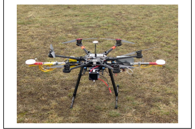
Figure 2. The DJI S800 UAV equipped with the multi-sensor system for DG. UAV: unmanned aerial vehicle; DG: direct georeferencing.
